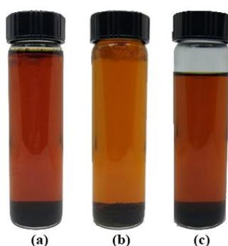
Figure 3. (a) Upgraded bio-oil without catalyst (b) Bio-oil upgraded with chemically activated vermiculite and (c) Bio-oil upgraded with physically activated vermiculite.
