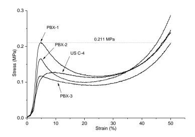
Figure 1. Curve of stress-strain of the explosive samples at a rate of 10 mm/min.
