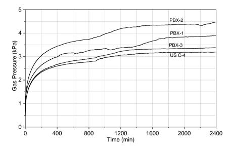
Figure 2. Curves of the relation between gas pressure and heating time by vacuum stability test at 100 °C for 40 hours.
