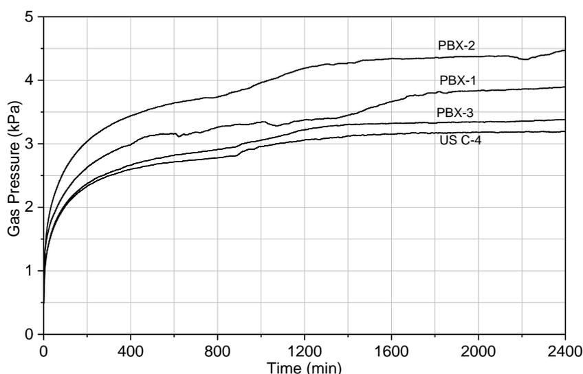
Figure 2. Curves of the relation between gas pressure and heating time by vacuum stability test at  $100^\circ\text{C}$  for 40 hours.
