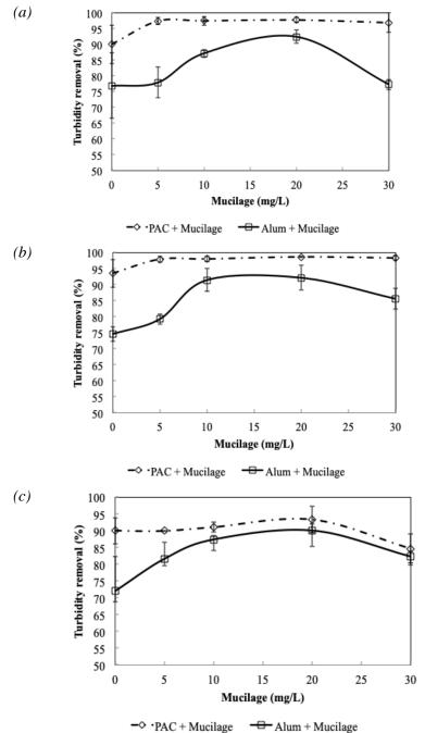
*Figure 4*. Turbidity removal by mucilage (BAM) in combination with PAC or alum at dosages of (a) 100 mg/L, (b) 120 mg/L, (c) 150 mg/L).
