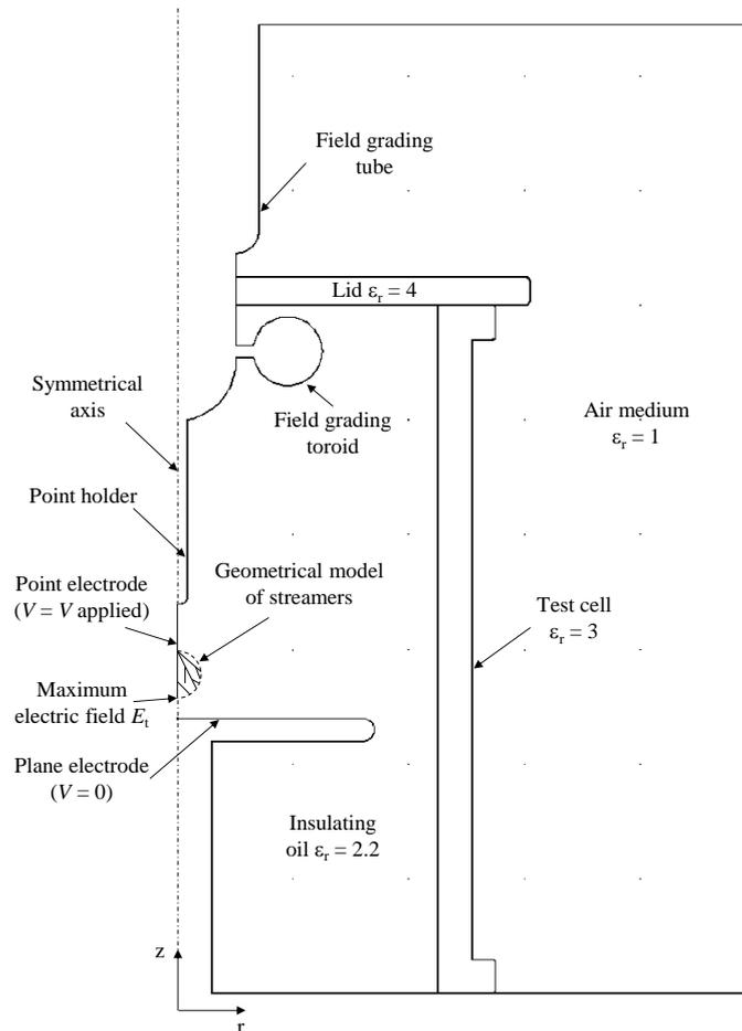
Figure 3. The 2D axial symmetry model for simulation of electric field distribution.
