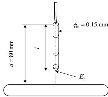
Figure 7. The model of growing cylinder for determination of electric field during streamer propagation in oil at 270 kV.
