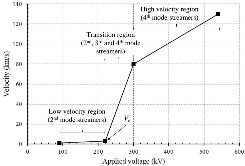
Figure 1. Positive streamer velocity versus applied voltage (redrawn from [6]).
