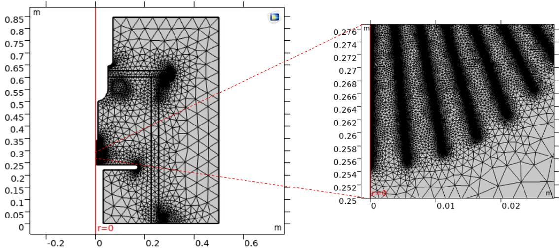
Figure 10. The mesh of the model for simulation of shielding effect ( $\phi = 75$  mm,  $\alpha = 5^\circ$ ).
