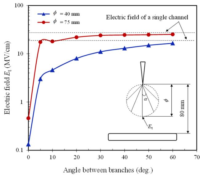
Figure 16. The channel tip field versus angle between branches.
