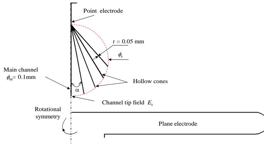
Figure 9. The 2D axial symmetry model for simulation of shielding effect with spherical model.
