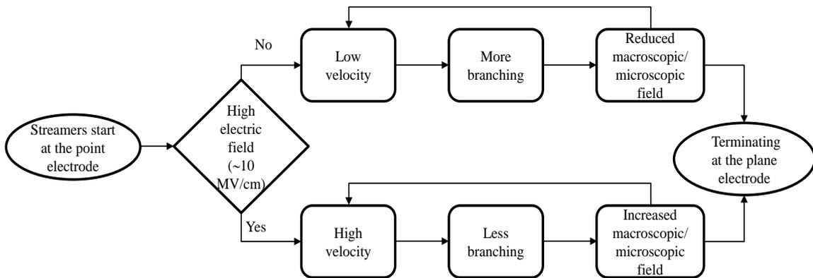
Figure 17. The diagram describing the correlation between branching and velocity of streamers.
