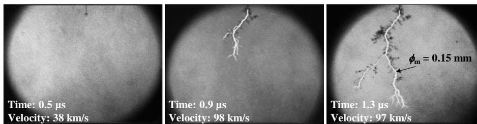
Figure 5. Images of the fast mode streamers (the 4<sup>th</sup> mode) in oil at 270 kV [6].
