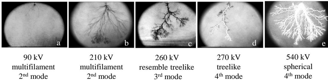
Figure 2. Streamer shape versus applied voltage [6].
