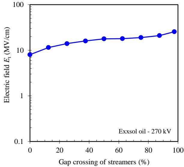
Figure 14. Channel tip field  $E_t$  versus streamer growth at 270 kV.
