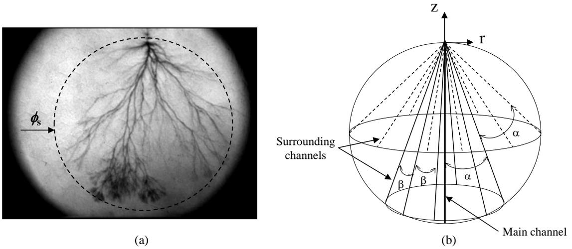
Figure 8. The image of the 2<sup>nd</sup> mode streamers [6] and the distribution of streamer branches at 210 kV.
