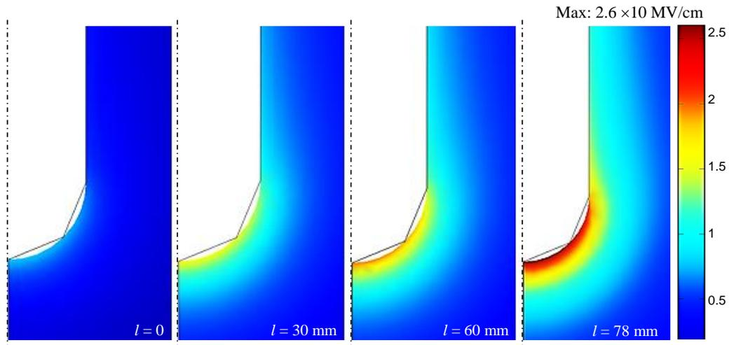
Figure 13. Distribution of the electric field around streamer channel tip at 270 kV.
