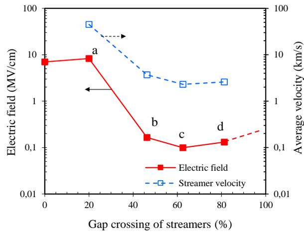
Figure 12. Velocity versus electric field at the channel tips of streamers at 210 kV.
