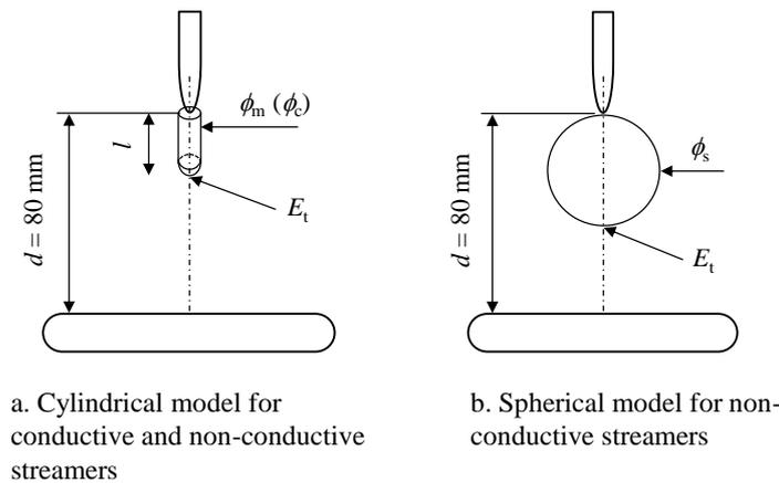
Figure 6. Models for simulation of electric field; (a)- $l = 16$  mm and  $\phi_m = 0.2$  mm for streamers in Fig. 4a,  $l = 37$  mm and  $\phi_c = 23$  mm for streamers in Fig. 4b; (b)- $\phi_s = 50$  mm and 65 mm for streamers in Fig. 4c and d.
