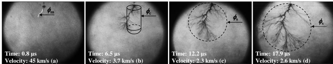
Figure 4. Framing images of streamers during propagation at 210 kV [6].
