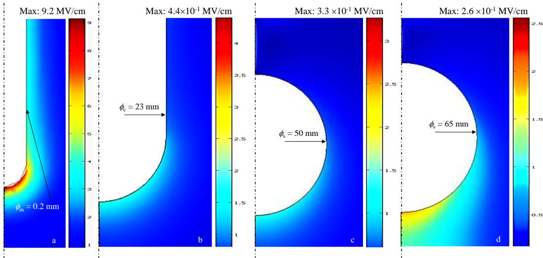
Figure 11. Plots of electric field. The letter symbols referred to streamer images shown in Fig. 4.
