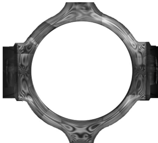
Figure 6. Isochrones field of the connecting-rod big end bearing.
