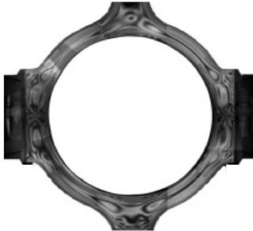
Figure 12. Isochrones field of the connecting-rod big end bearing at static situation,  $0^\circ$  of crankshaft angle.
