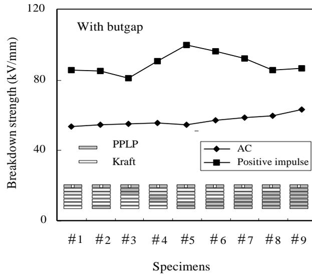
Figure 8. Breakdown strength of PPLP/Kraft for the with butt gap samples.
