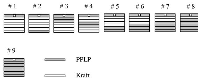
Figure 2. PPLP and Kraft layer configuration for the with butt gap samples.
