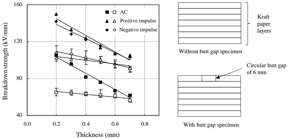
Figure 5. Breakdown strength versus thickness of Kraft. Full symbols for without butt gap; open symbols for with butt gap samples.
