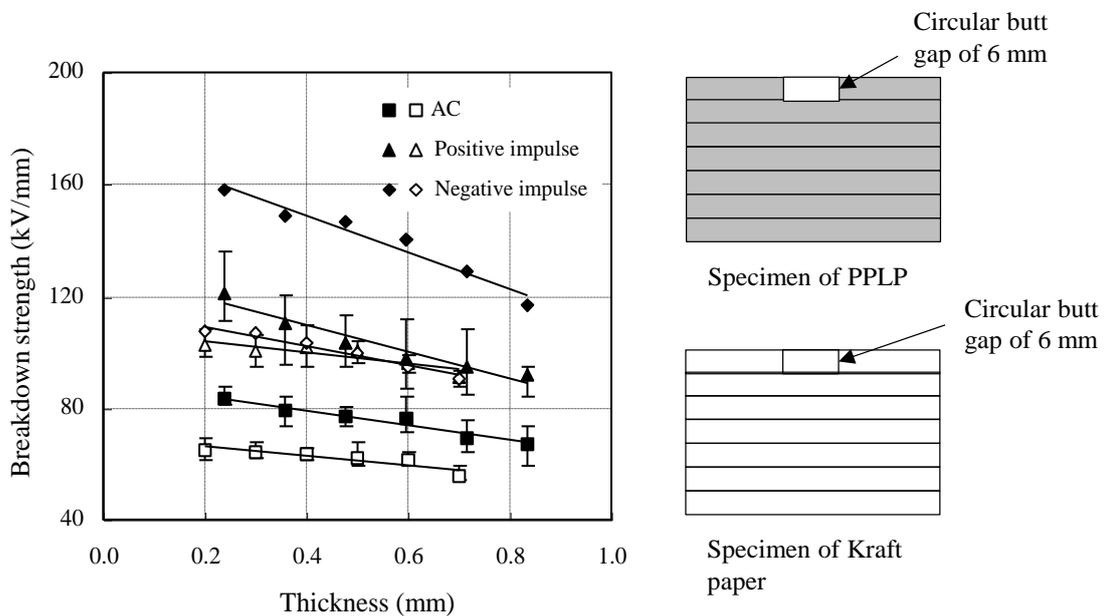
Figure 6. Breakdown strength comparison. Full symbols for PPLP; open symbols for Kraft samples.
