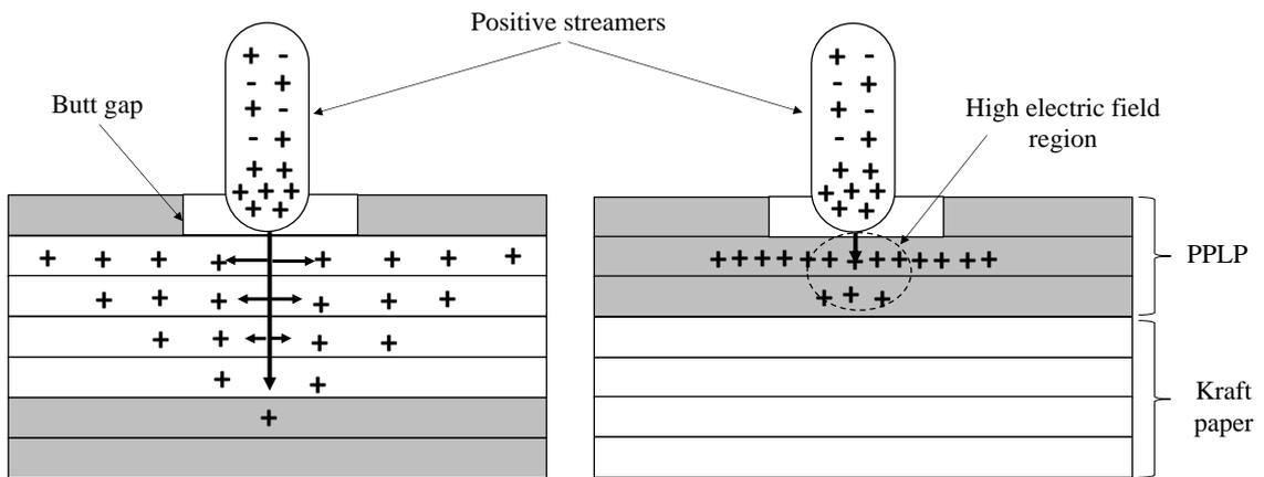
Figure 9. Charge accumulation on PPLP
