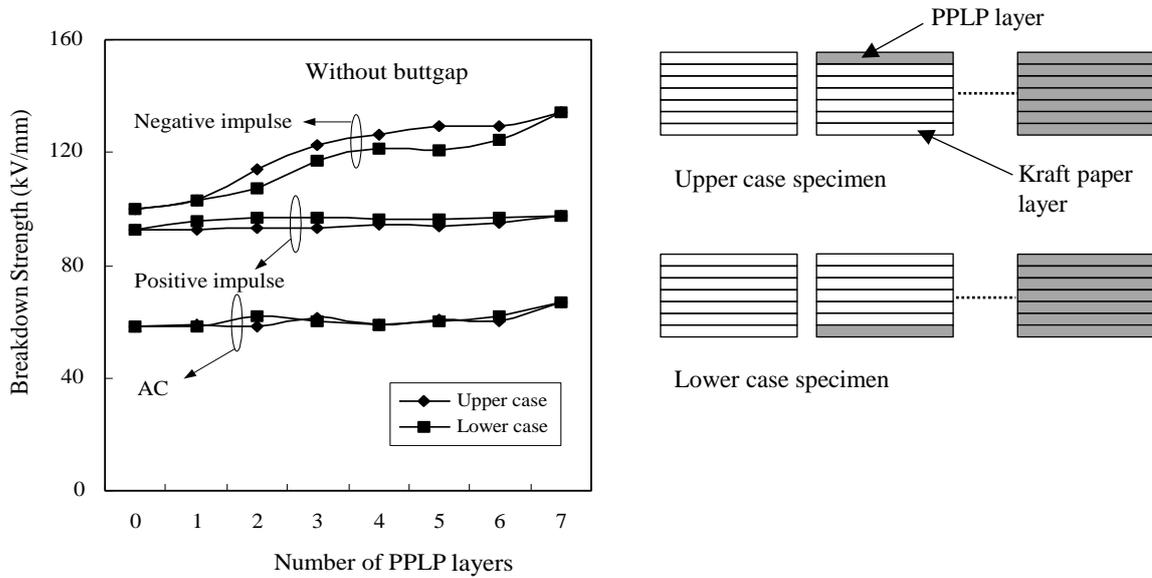
Figure 7. Breakdown strength of PPLP/Kraft for the without butt gap samples.
