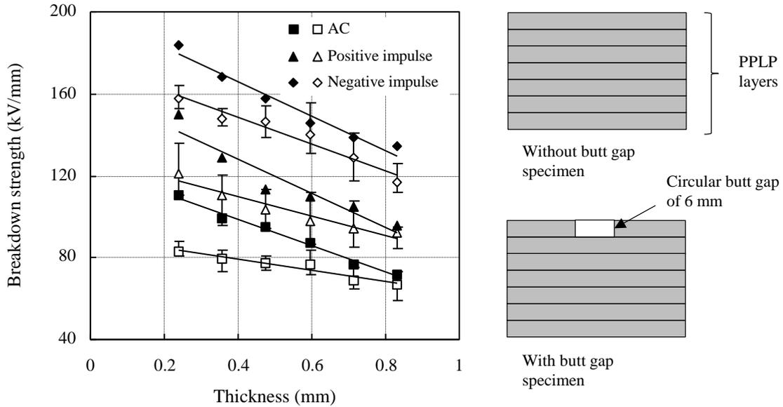
Figure 4. Breakdown strength versus thickness of PPLP. Full symbols for without butt gap; open symbols for with butt gap.
