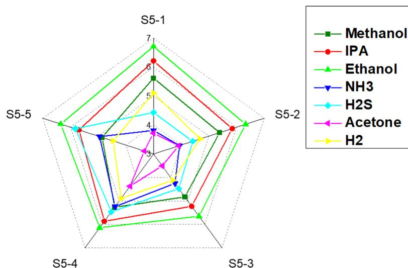
Figure 5. Radar plot of sensor responses of five sensor elements in the array gas sensor in a static system when exposed to volatiles of Methanol, IPA, Ethanol, Ammonia, Hydrogen sulfide, Acetone, and Hydrogen at power of 165 mW.
