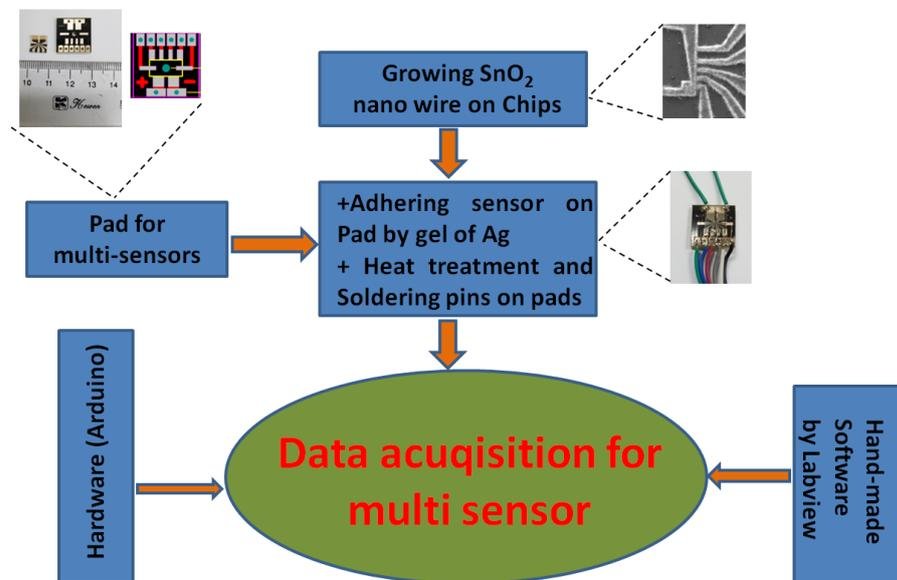
Figure 1. Flow chart for  $\text{SnO}_2$  nanowires-based array gas sensor.
