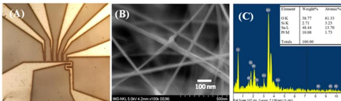
Figure 2. (A) Low and (B) high magnification SEM images of the array sensor; (C) EDX showing the elements present in the decorated  $\text{SnO}_2$  nanowires.
