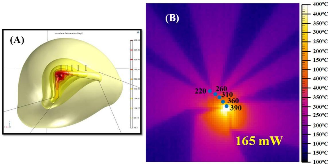
Figure 3. Gradient temperature (A) simulation on COMSOL, and (B) Infrared Emission Image on chip.
