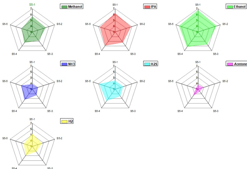
Figure 6. Enclosed area extracting from radar plot for the sensor array at power of 165 mW.
