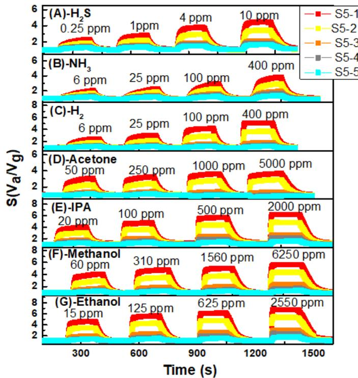
Figure 4. Gas sensitivity at power of 165 mW when exposed to (A) H<sub>2</sub>S, (B) NH<sub>3</sub>, (C) H<sub>2</sub>, (D) Acetone, (E) IPA, (F) Methanol, (G)-Ethanol with different concentrations.
