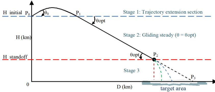
Figure 2. Maximum range trajectory scheme for UFVs.
