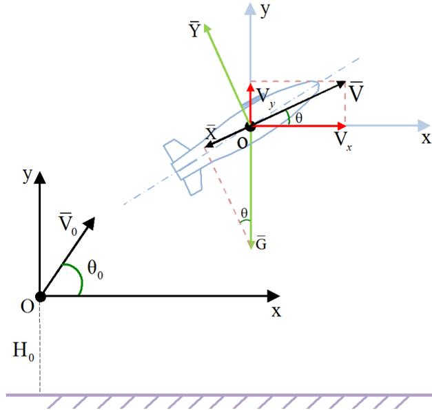
Figure 1. Diagram of forces acting on the center of mass of UFVs.
