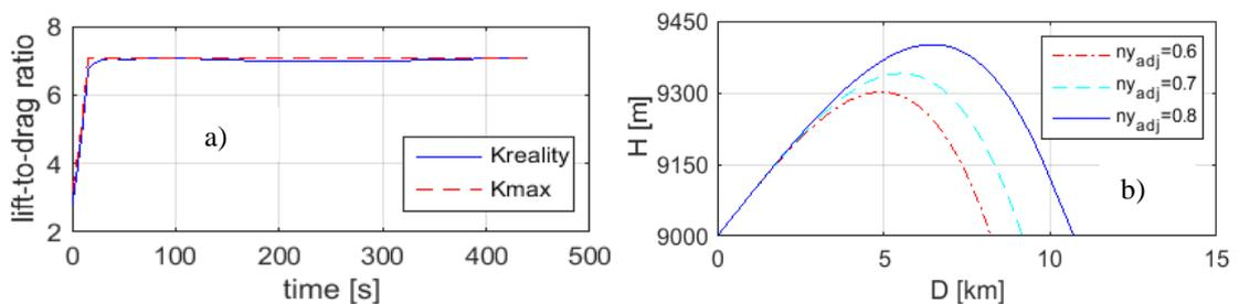
Figure 8. Lift-to-drag ratio (a) and trajectory expansion section (b).
