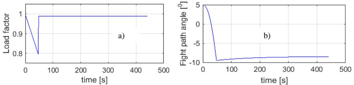
Figure 6. Normal load factor (a) and flight path angle (b).
