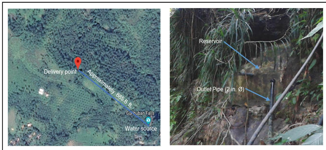
Figure 2. The distance between the source and the village (left) and the actual situation of the water source (right).
