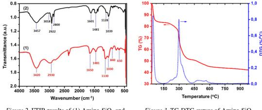
*Figure 2.* FTIR results of (1) Amine-SiO<sub>2</sub> and (2) Akualite A420.
