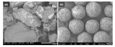
Figure 1. SEM images of (a) Amine-SiO<sub>2</sub> and (b) Akualite A420.
