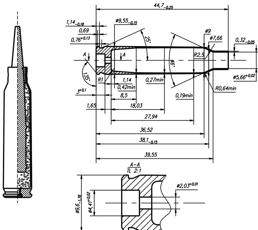
Figure 4. The parameters of 5.56 mm underwater cartridge.
