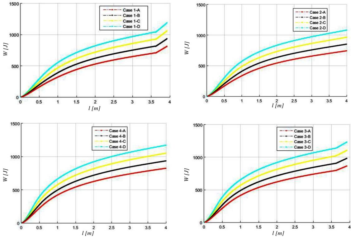
Figure 6. The total energy conversion vs. trajectory of projectile.
