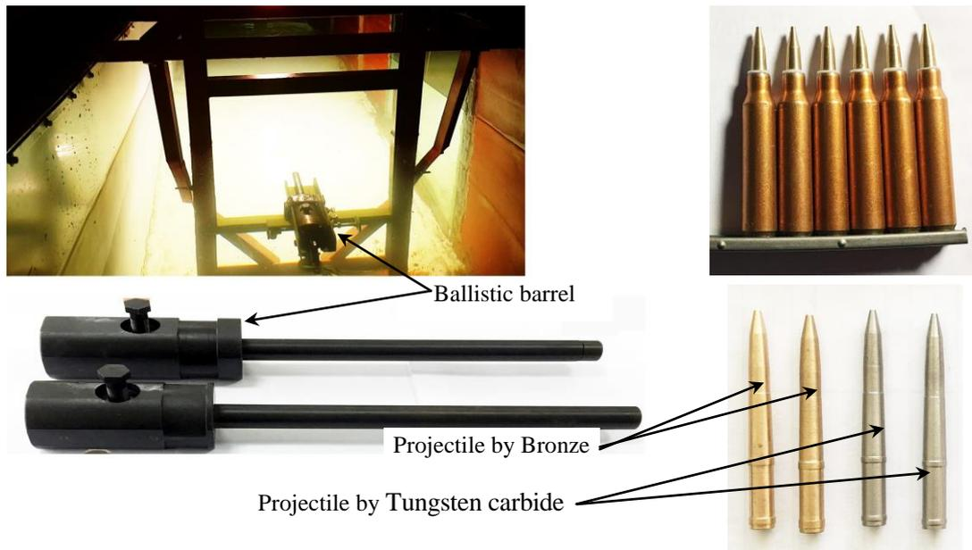
Figure 10. Schematic of the experimental setup with the ballistic barrel.
