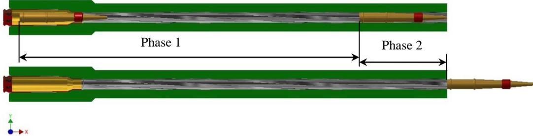
Figure 2. Schematic of the process of the underwater projectile move in the barrel.
