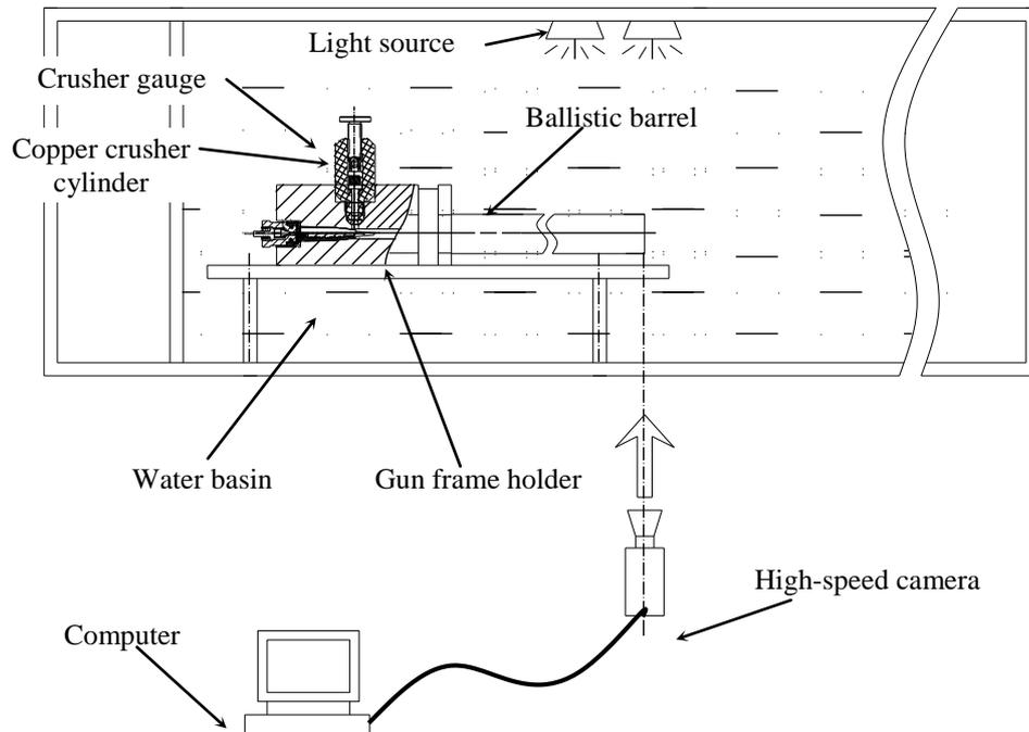
Figure 9. Schematic of the experimental setup.
