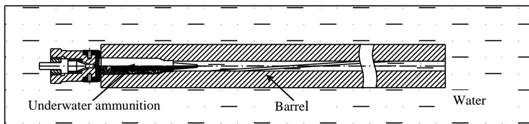
*Figure 1. The brief models of underwater projectile move in the barrel.*
