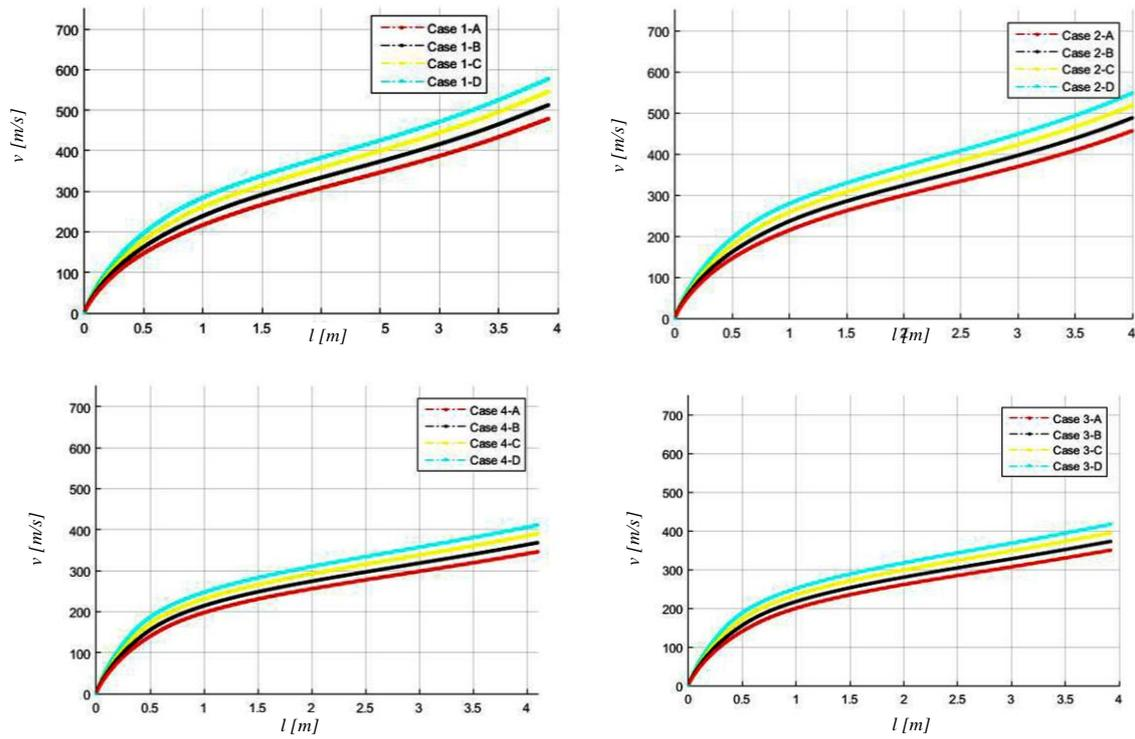
Figure 8. The muzzle velocity vs. trajectory of projectile.
