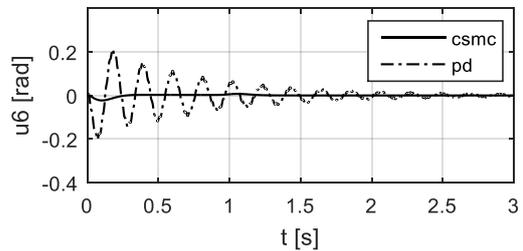
Figure 10. Slope deflection at the right end of the link: CSMC vs. PD.
