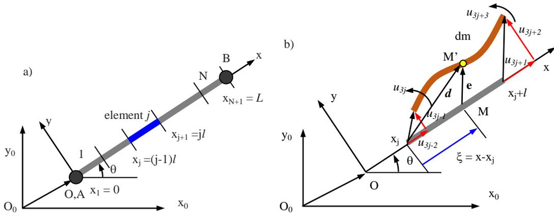
Figure 1. (a) Configuration diagram of a link of manipulator. (b) Typical  $j^{\text{th}}$  finite element of the link in the floating frame  $Oxy$  and the fixed frame  $O_0x_0y_0$ .
