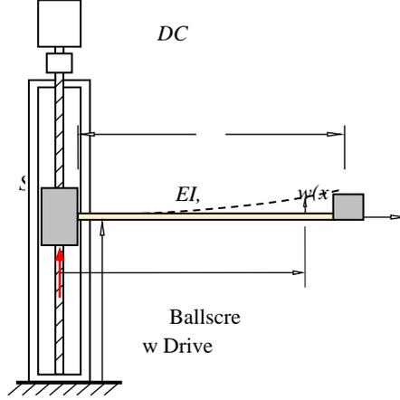
Figure 2. Flexible Cartesian manipulator.
