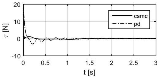
Figure 7. Control force: CSMC vs. PD.
