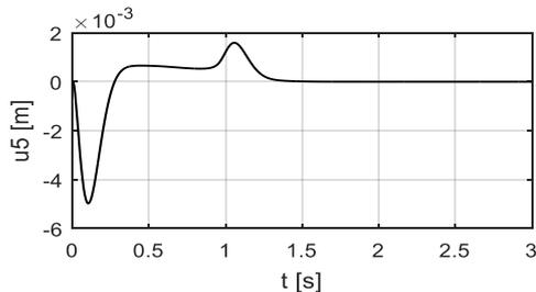
Figure 5. Transverse deflection at the right end of the link.
