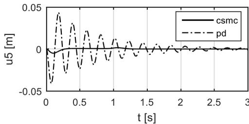
Figure 9. Transverse deflection at the right end of the link: CSMC vs. PD.
