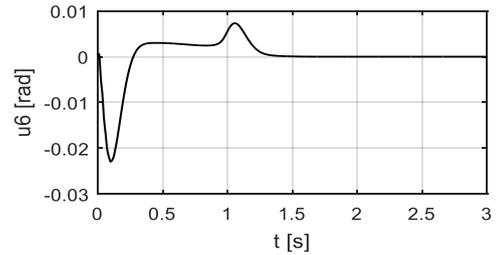
Figure 6. Slope deflection at the right end of the link.
