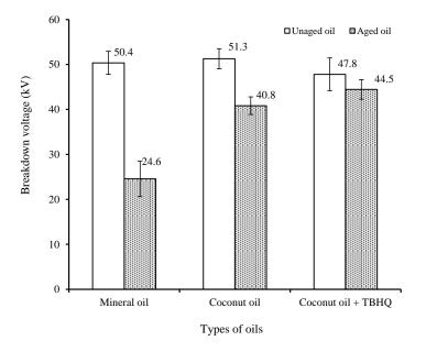
*Figure 2.* Breakdown voltages of oil samples (d = 2.5 mm).
