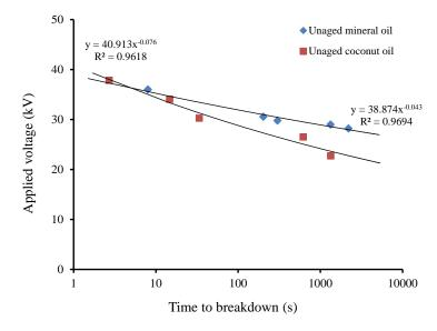
*Figure 4. V-t* plots of oil samples (d = 2.5 mm).
