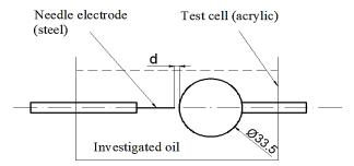
b. Needle-sphere electrode system
