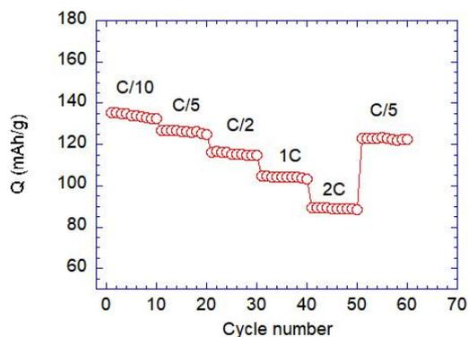
Figure 6. Rate capability test of NFC-1 cathode material.
