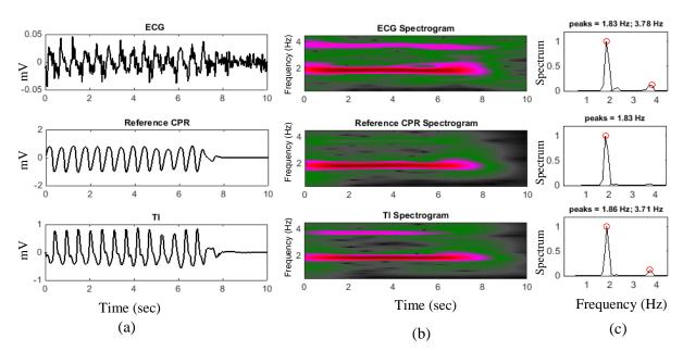
*Figure 2.* Signals, corresponding frequency distributions, and spectrograms of (a) ECG, Reference CPR, and TI signals. (a) Signals in time domain; (b) Gabor Spectrograms; (c) Frequency distributions. The reference CPR in this segment is with 1.83 Hz, approximate to 110 compressions per minute (cpm), coincided with that in the ECG, and close to TI frequency.
