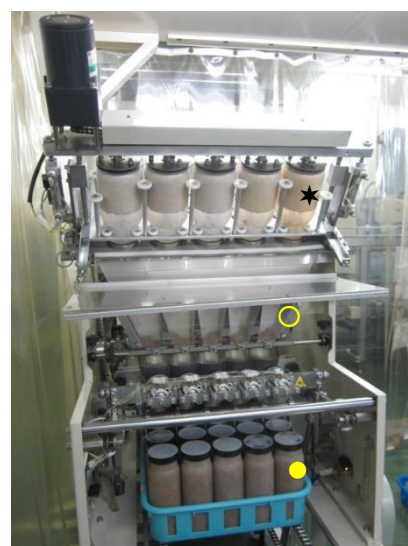
Figure 10: Inoculation machine for solid spawn. (★: solid spawn, ○: stainless slide, ●: sterilized medium in P.P. cultivation bottle) (Photo by Dr. K. Yamanaka).
