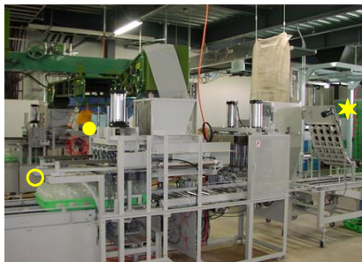
Figure 7. Filling machine for P.P. bottle cultivation. (★: P.P. cap, ○: empty P.P cultivation bottle, ●: medium filling).
