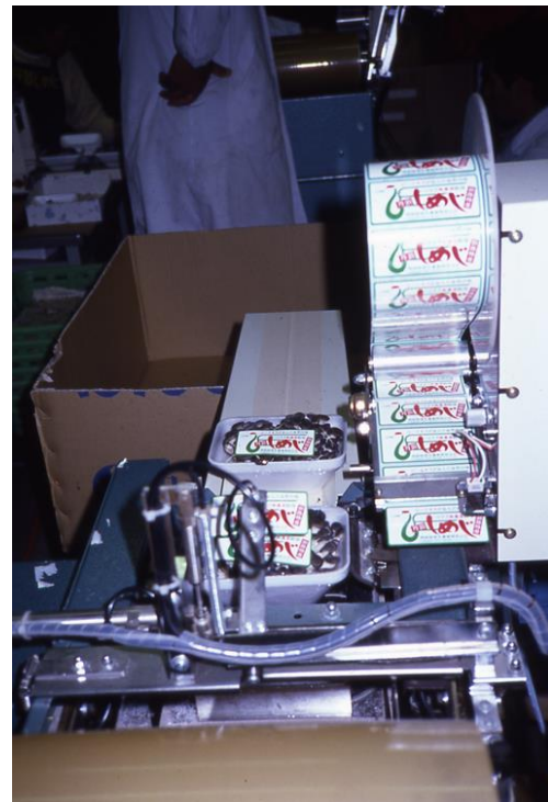
Figure 22. Wrapping machine for Pleurotus ostreatus . (Photo by Dr. K. Yamanaka).
