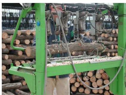
Figure 1. Drilling of wood-log for the inoculation of plug spawns. (Photo by Mr. Nakazawa).
