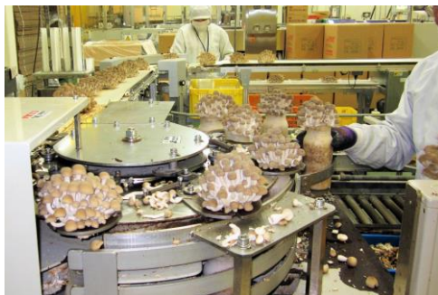
Figure 21. Automated cropping of Hypsizygus marmoreus . (Photo by Dr. K. Yamanaka).
