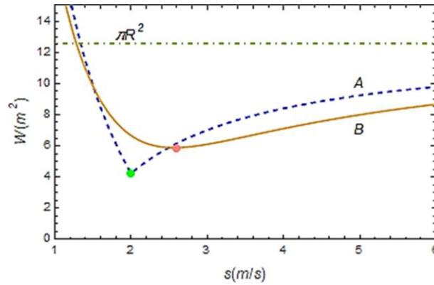
*Figure 2.* The  $s$  dependence of the total wetness on turbine blades in case of swept space in cylindrical (curve A with dashed line) and ellipsoid shape (curve B with solid line).
