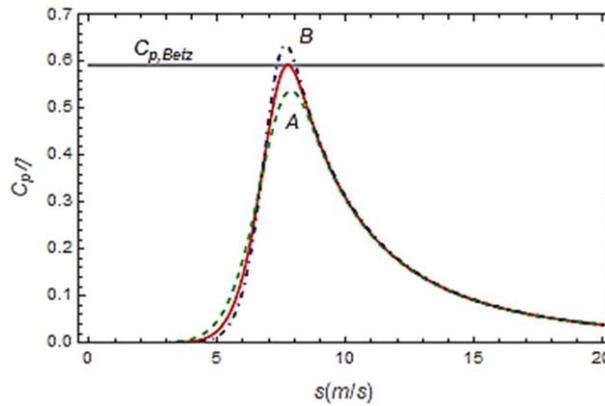
Figure 3. The  $s$  dependence of power coefficients is plotted with  $\lambda = 7$  m/s and three different values of shape parameters:  $\kappa = 8$  (dashed line), 10 (solid), and 12 (dot-dashed) for the lines from A to B.
