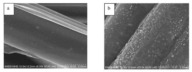
Figure 2. SEM image of non-woven fabric without (a) and with AgNPs (b) incorporated.
