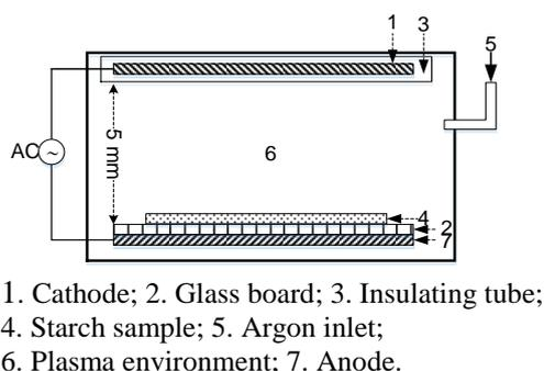
1. Cathode; 2. Glass board; 3. Insulating tube;
