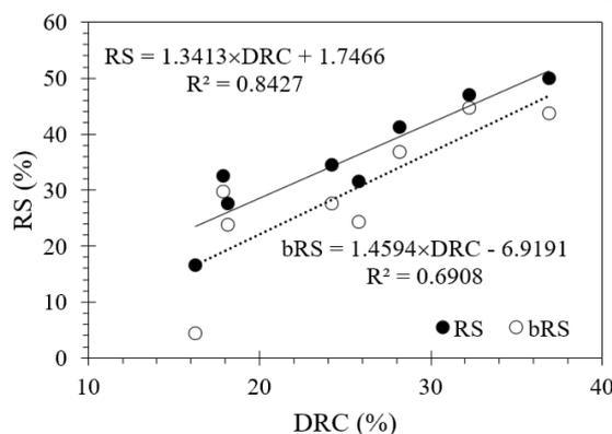
Figure 7. The relationship between relative crystallinity (DRC) and resistant starch fraction of samples without (RS) or with (bRS) pre-boiling before digestibility measurement.
