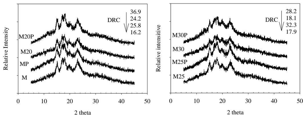
Figure 6. X-ray diffraction patterns and relative crystallinity (DRC, right-upper values) of samples (M: raw starch; M20, M25 and M30: HMT starches at 20, 25 and 30 % moisture content; P: plasma treated starches).
