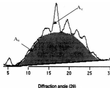
Figure 2. The calculation of degree of relative crystallinity (DRC).
