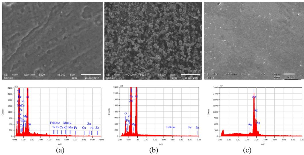
Figure 1. Photo of SEM and EDX spectrum on surface of A6061 pattern (a); zincatized A6061 pattern (b); silver plating A6061 pattern.
