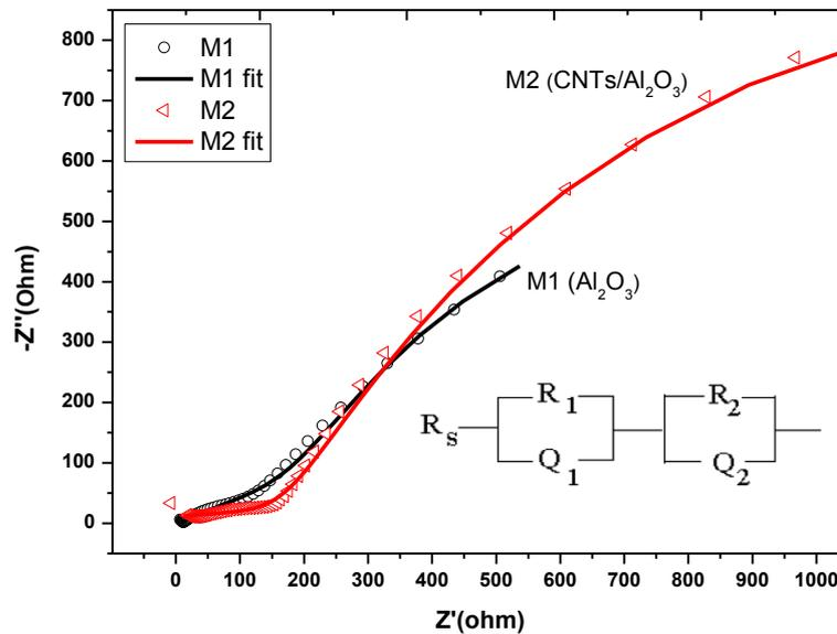
Figure 7. Nyquist diagram of  $Al_2O_3$  and CNTs/ $Al_2O_3$  coating measured in 3.5 % NaCl solution.
