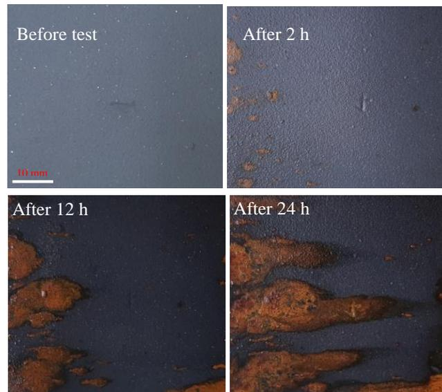
*Figure 4.* Surface change of Al<sub>2</sub>O<sub>3</sub> coating during the salt spray test.
