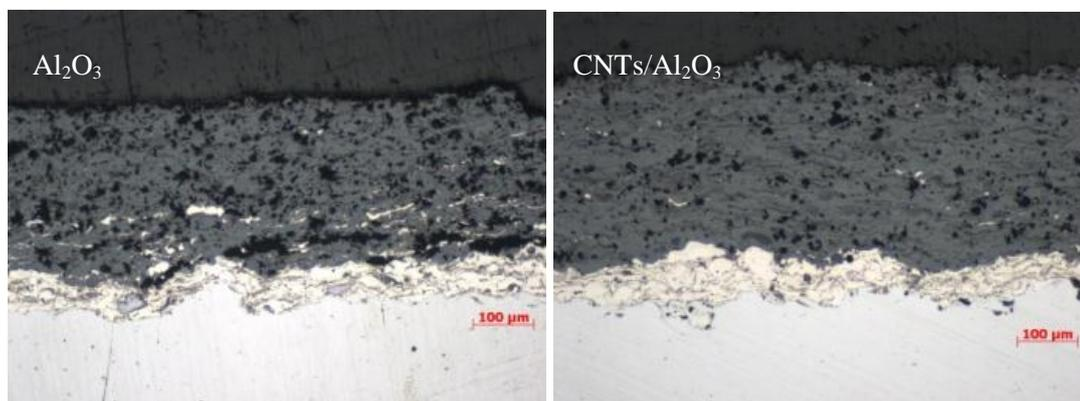
Figure 6. Cross-sectional structures of  $\text{Al}_2\text{O}_3$  and  $\text{CNTs}/\text{Al}_2\text{O}_3$  coatings.
