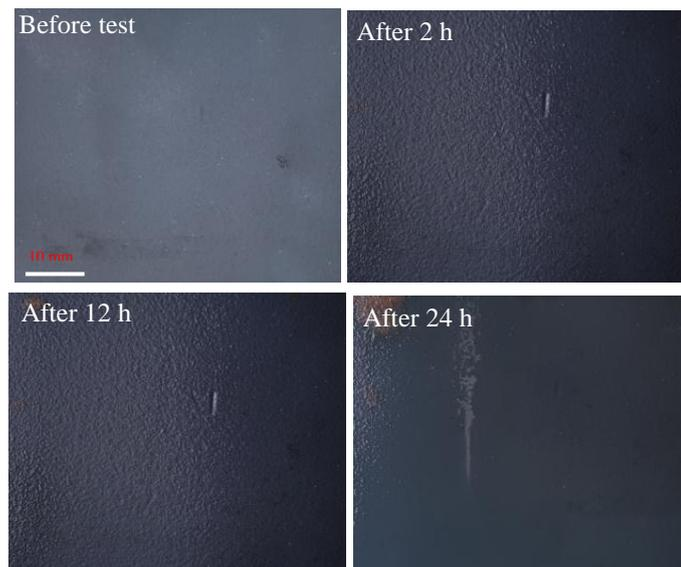
*Figure 5.* Surface change of CNTs/Al<sub>2</sub>O<sub>3</sub> coating during the salt spray test.
