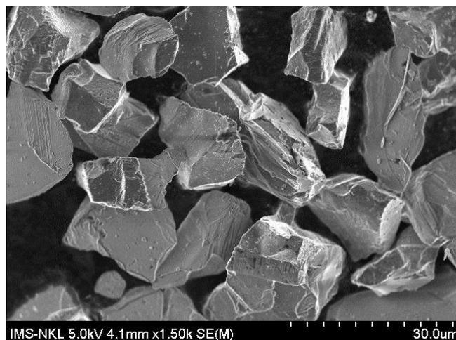
*Figure 1.* SEM image of Al<sub>2</sub>O<sub>3</sub> powder before mixing with CNTs.
