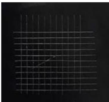
Figure 5. Aspect of the Zr/Ti/MoCC-ED coating sample after the tape adhesion tests .
