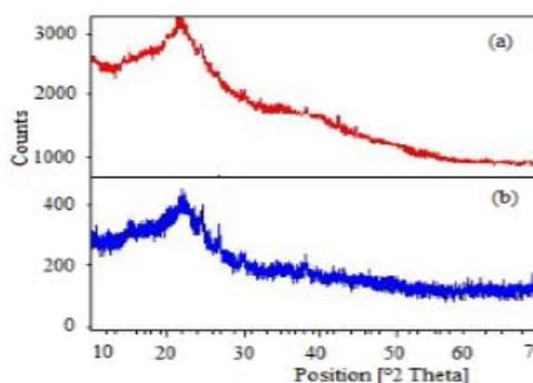
Figure 4. XRD of (a) coffee husk, (b) biochar.
