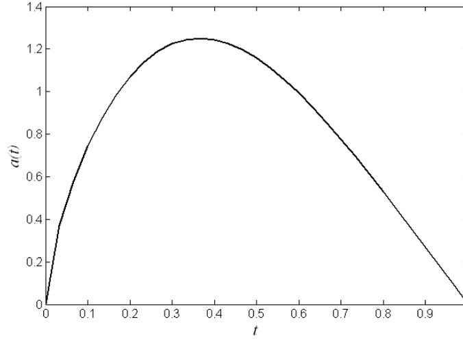
Figure 3. The column's optimal shape
