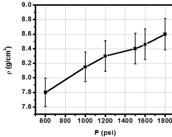
Figure 3. The dependence of the magnet mass density  $\rho$  on the compaction pressure  $P$ .
