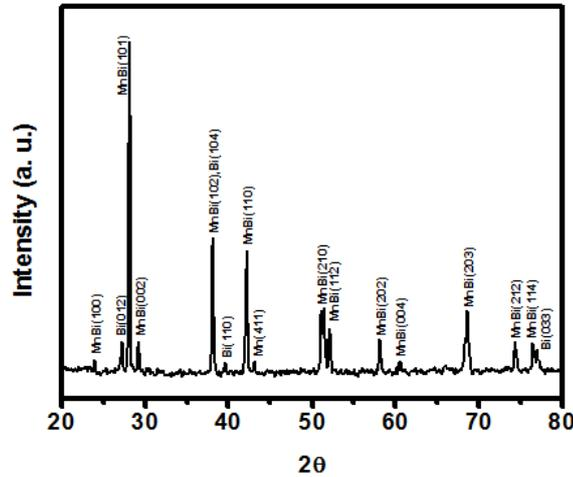
Figure 1. PXR pattern of the sample  $Mn_{50}Bi_{50}$  alloyed by arc-melting and annealed at 300 °C superimposed by  $gradT = 2$  °C/cm. The sample was finely ground to avoid any effect of the crystalline texture.
