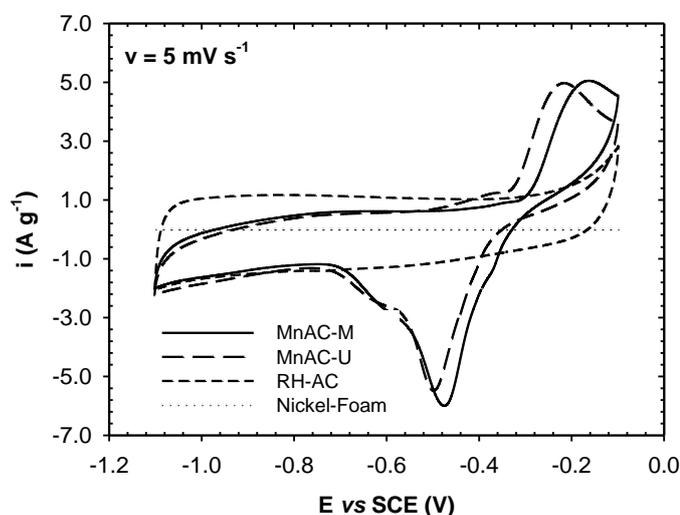
Figure 7. CV of RH-AC and MnAC electrodes in 6M KOH electrolyte at scan rate of  $5 \text{ mV s}^{-1}$ .
