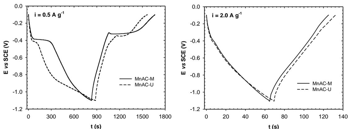
Figure 9. Galvanostatic charge-discharge curves of MnAC-M and MnAC-U at current densities of 0.5 and 2.0 A g<sup>-1</sup>.
