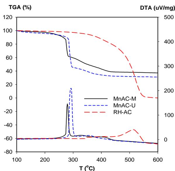
Figure 2. TGA thermograms of RH-AC and MnAC samples.
