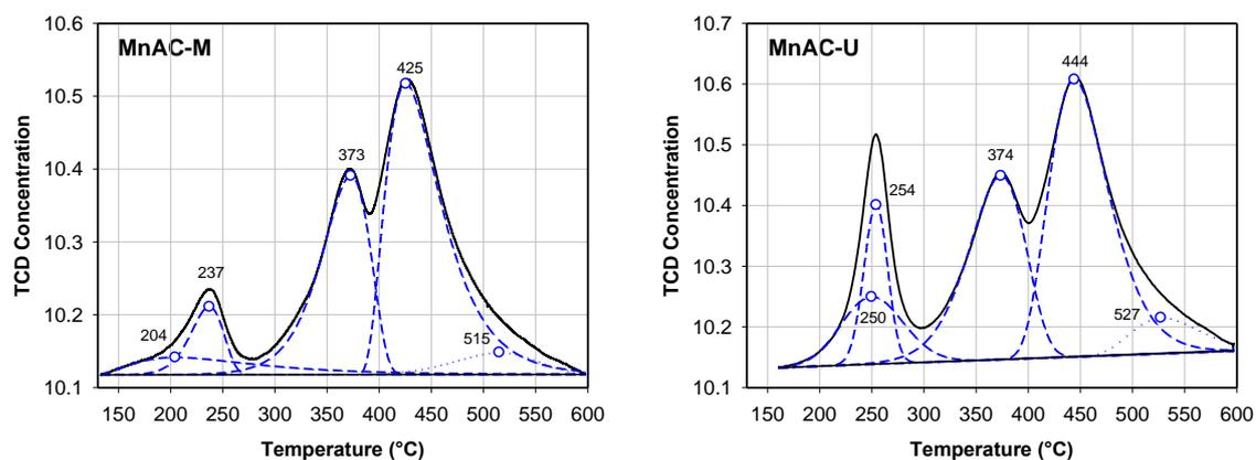
Figure 4. Deconvolution of TPR-H<sub>2</sub> profile of MnAC samples.
