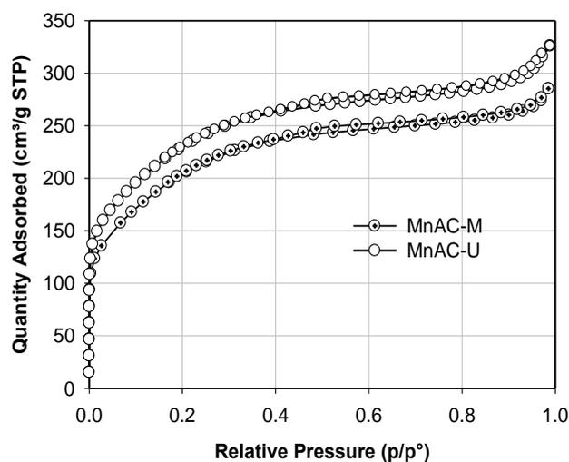
Figure 6. Nitrogen adsorption – desorption isotherms of MnAC samples.
