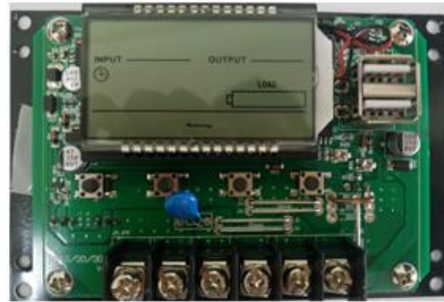
Figure 9. Solar controller board.
