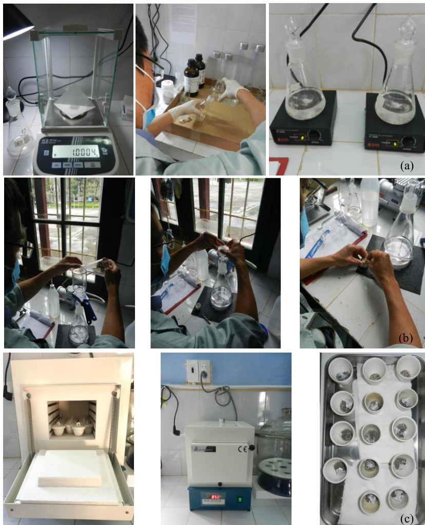
Figure 6. Procedure of the hydration reaction test: (a) 1 g of dried sample was precisely obtained, mixed with a compound solution, and agitated by a magnetic stirrer in the stoppered Erlenmeyer flask; (b) a suction filtration separated the mixture, and the residues together with the filter paper were put into a crucible, (c) the residues were heated at 850°C for one hour before weight measurement
