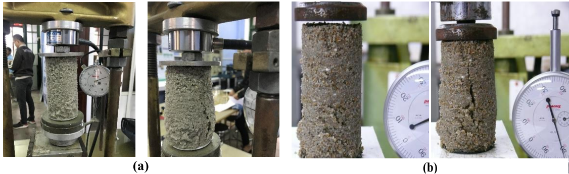
Figure 5. Photos of typical unconfined compression tests on specimens of (a) GBFS specimen and sand-GBFS mixtures
