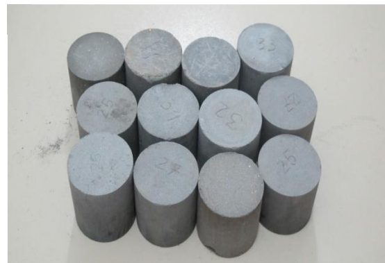
Figure 3. Lightweight materials were fabricated following the lime + pozzolan binder
