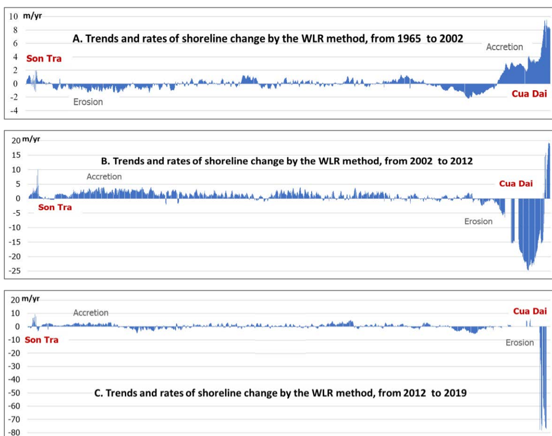
Figure 10. Trends and rates of shoreline change in Son Tra - Cua Dai area by the WLR method, in the periods: (a) from 1965 to 2002; (b) from 2002 to 2012 and (c) from 2012 to 2019
