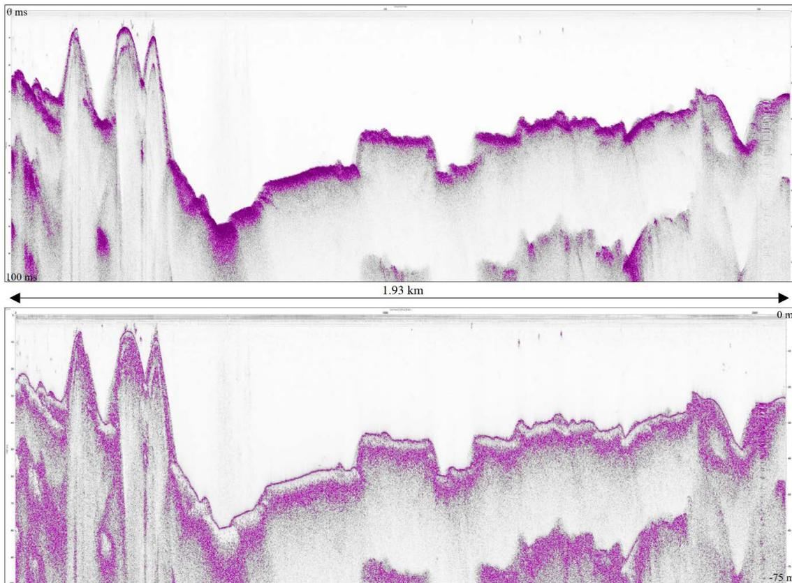
Figure 5. Cross-section of HRSP MC03 before (top) and after processing (bottom)
