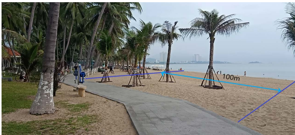
Figure 2. Sampling design: the width is measured from the low tide waterline to the concrete embankment area above the beach
