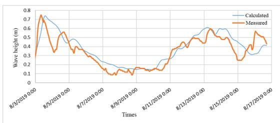
Figure 6. Comparison of wave height data measured and calculated results
