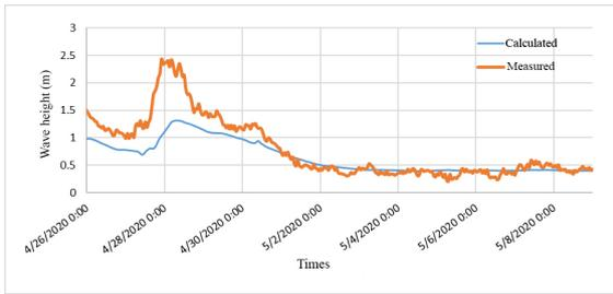
Figure 10. Comparison of wave height data measured and calculated results
