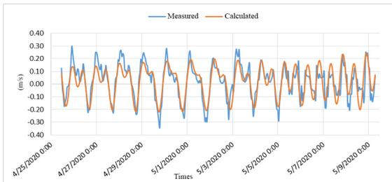
Figure 12. Comparison of U flow velocity components measured and calculated results
