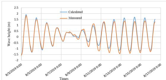
Figure 4. Comparison of measured water level data with calculated results
