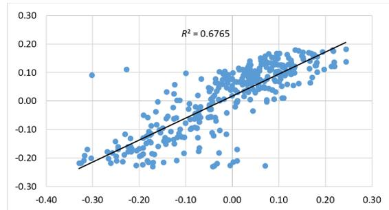
Figure 15. Correlation of V flow velocity components measured and calculated results
