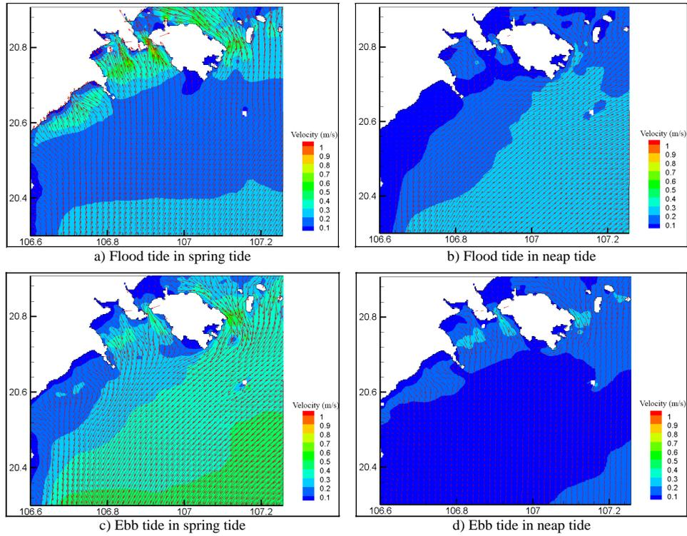
Figure 18. Detailed currents field in the study area under scenario 1
