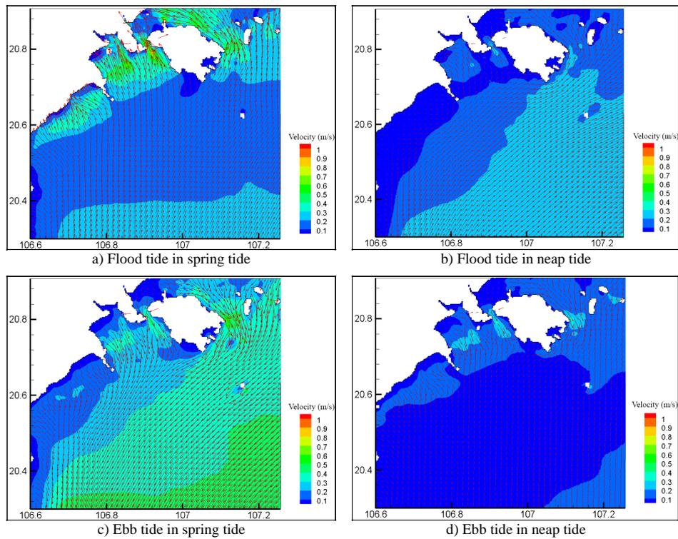
Figure 19. Detailed currents field in the study area under scenario 2
