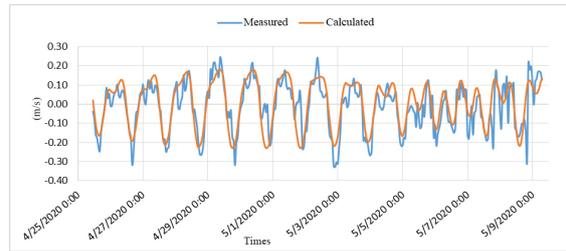
Figure 14. Comparison of V flow velocity components measured and calculated results
