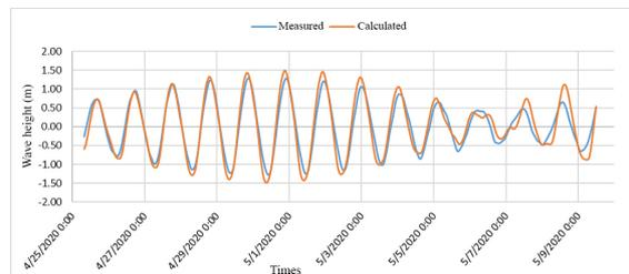
Figure 8. Comparison of measured water level data with calculated results
