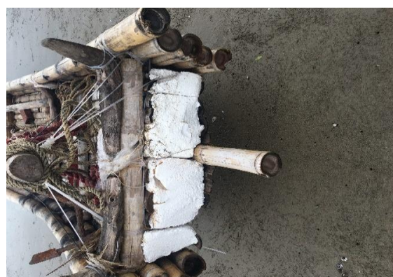
Figure 3a. Fishing boats are made of foam material
