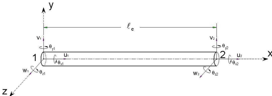
Figure 1. Three dimensions 2-node beam element model
