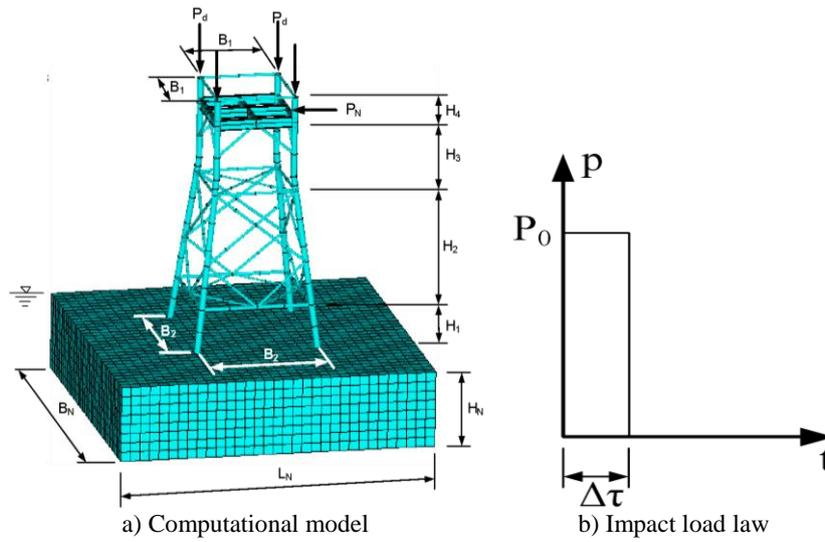
Figure 4. Computational model and impact load law
