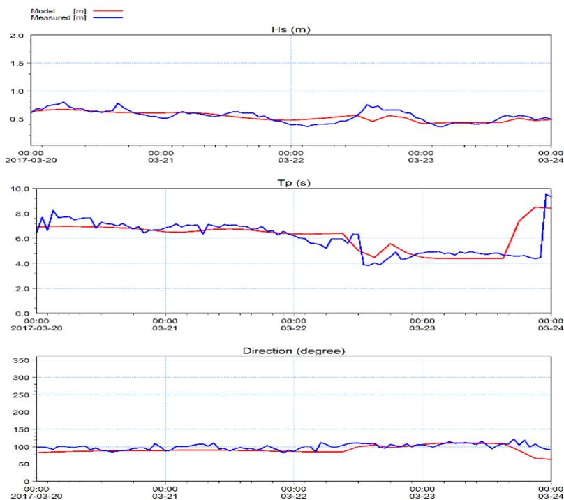
Fig. 4. Measured and calculated wave heights, wave periods and wave directions at AWAC station
