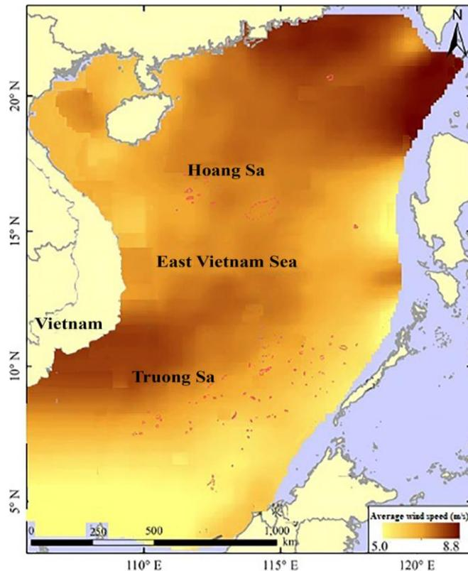
Figure 3. Average wind speed based on QuikSCAT data from 2006 to 2009 in the study area
