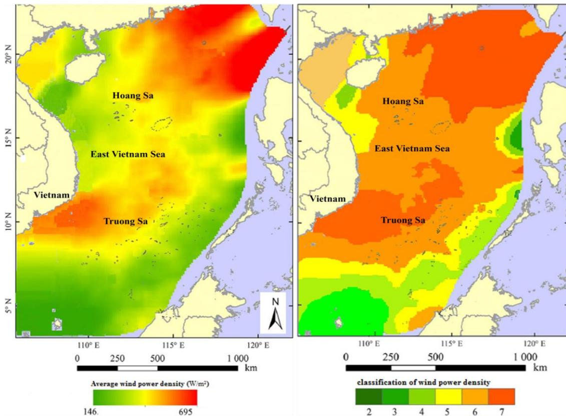
Figure 4. Average wind power density and classification of wind power density
