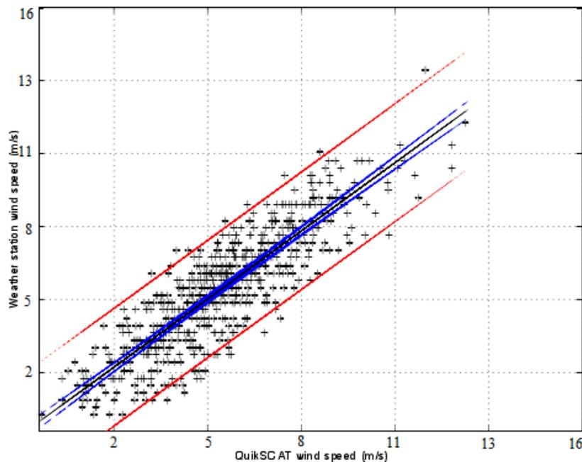
Figure 2. Scatter plot of observed wind speeds of QSCAT and Truong Sa island weather station after erroneous data pairs were removed. Black line is the linear regression. The blue and red lines are the 95% confidence level for the regression line and regression points, respectively
