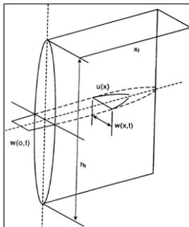
Fig.1. The PKN fracture geometry [10]
