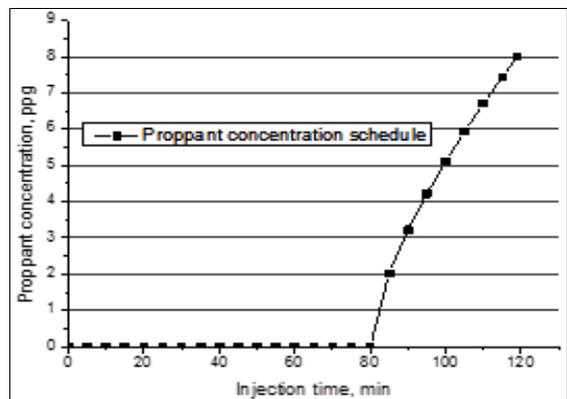
Fig. 5. Proppant concentration schedule during pumping
