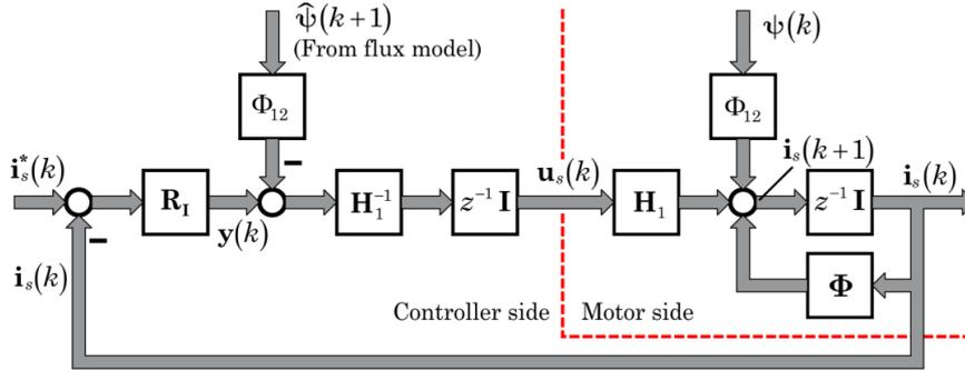
Figure 13: Block structure of the current vector controller for IM ([9])
