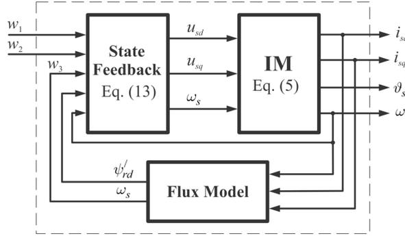
Figure 16: Substitute linear process model of the IM as starting point for controller design ([9])
