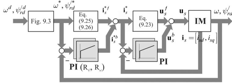
Figure 17: The block structure of the flatness-based IM control (concrete design steps can be seen in ([9])
