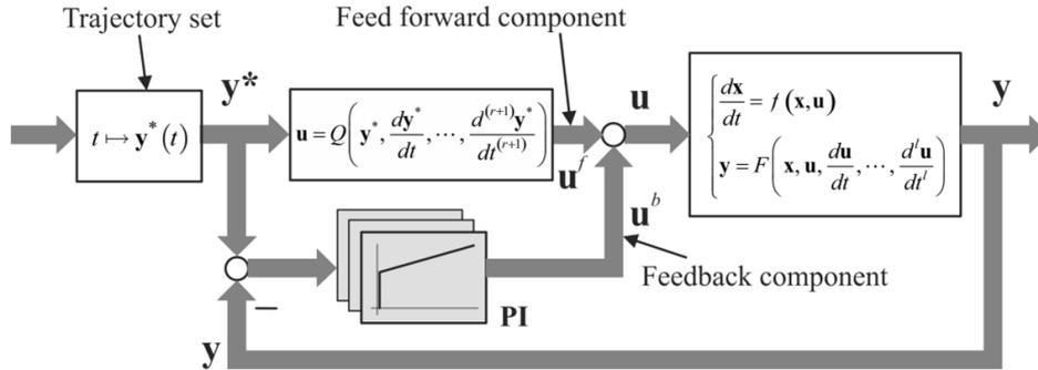
Figure 11: The general flatness-based control structure ([9])
