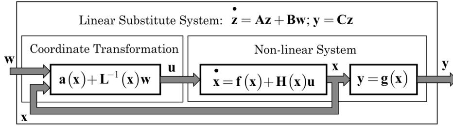
Figure 10: Concept of exact linearized process model ([9])
