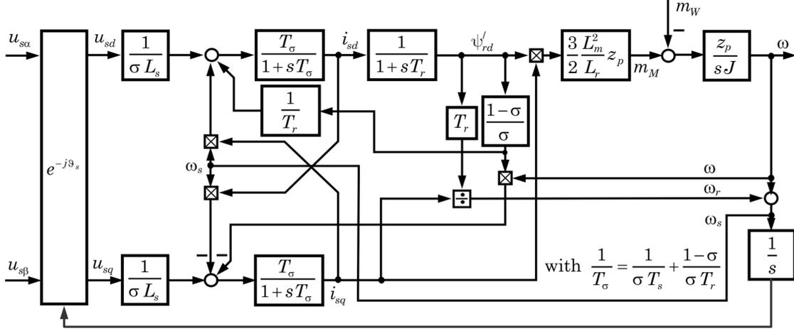
Figure 7: Model of the IM in field synchronous  $dq$  coordinate system
