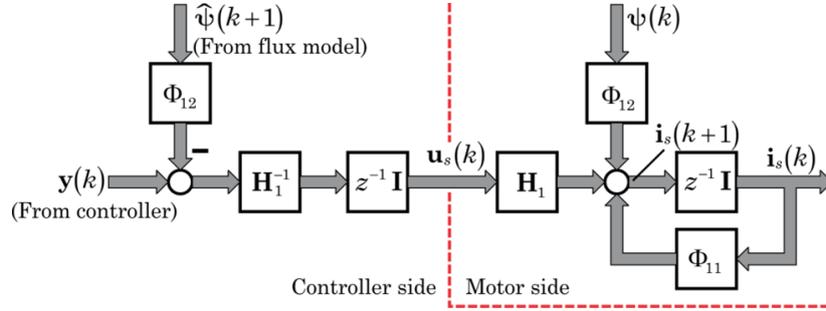
Figure 12: The general compensated process model  $\mathbf{i}_s$  ([9])
