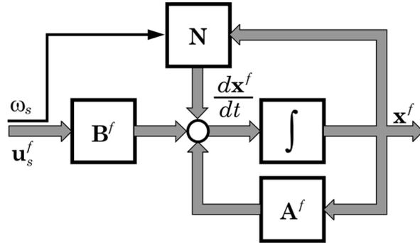
Figure 8: State space model of the IM in  $dq$  coordinates
