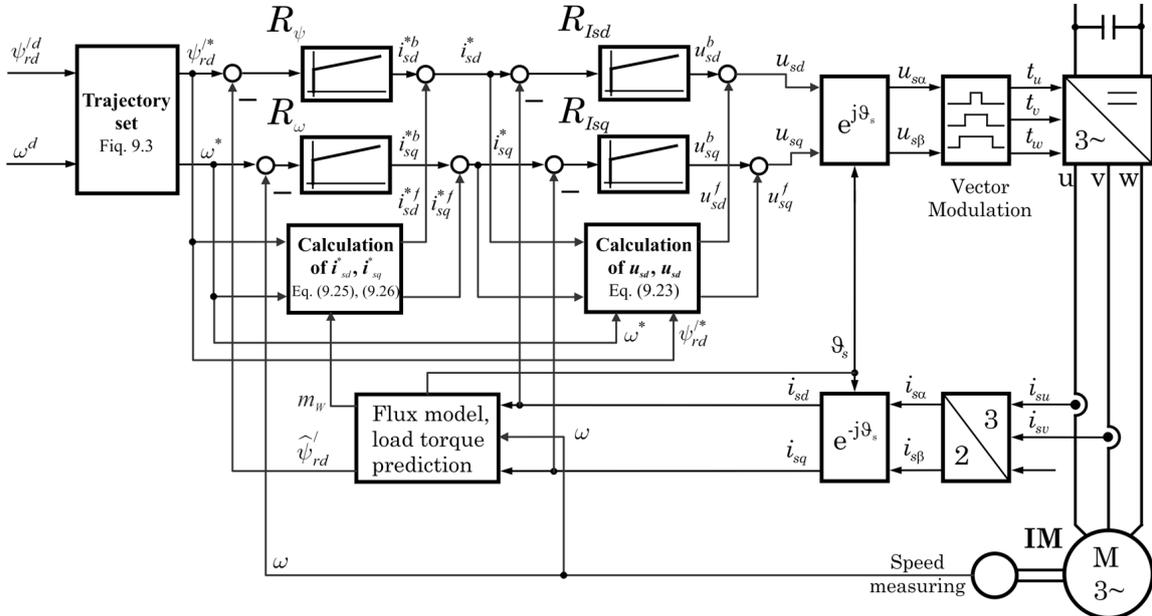
Figure 18: The detailed flatness-based cascaded control structure for IM drives ([9])
