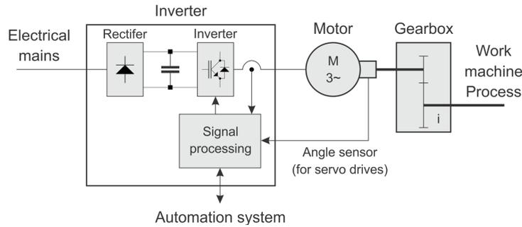
Figure 1: Structure of a drive system in the practice [8]
