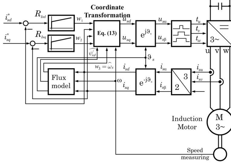
Figure 15: The new control structure of the inner loop with direct decoupling designed by using the method of exact linearization ([9])
