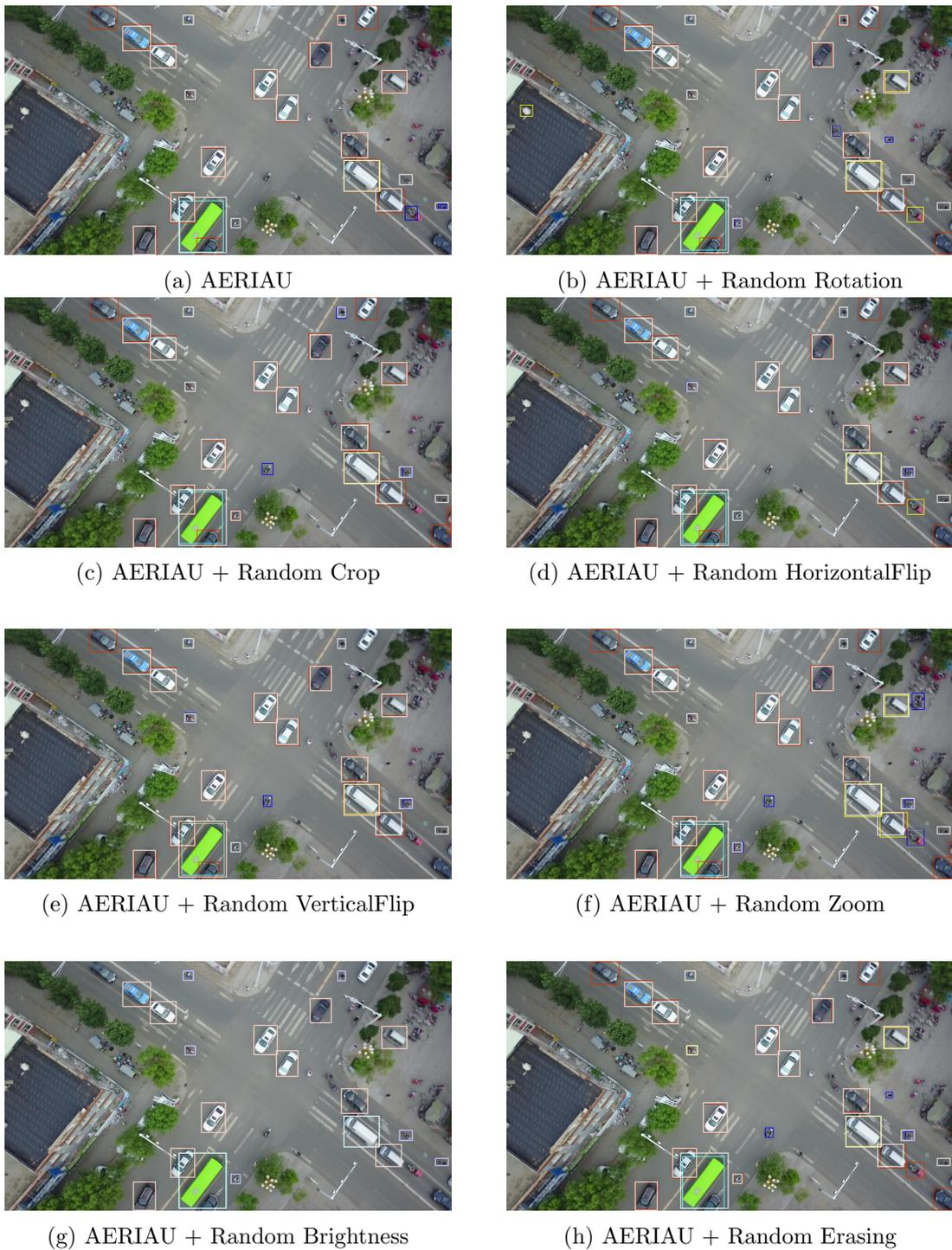
Figure 5: Faster RCNN: Visualization results of Single Data Augmentation Strategies. Color legend: truck, car, bus, motor, and Ground Truth.
