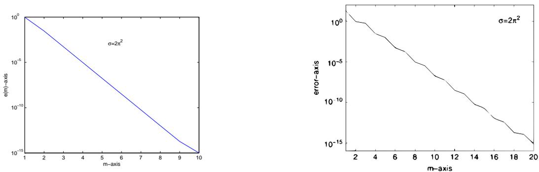
Figure 1. The errors  $e(m)$  of our Method DIM2 (left) vs. the Wang's fastest method (right) in Example 1 for  $k = 1, \sigma = 2\pi^2$
