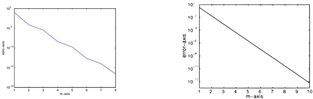
Figure 3. The errors  $e(m)$  of our Method DIM2 (left) vs. the Wang's fastest method (right) in Example 2 for  $k = 0.1$ .
