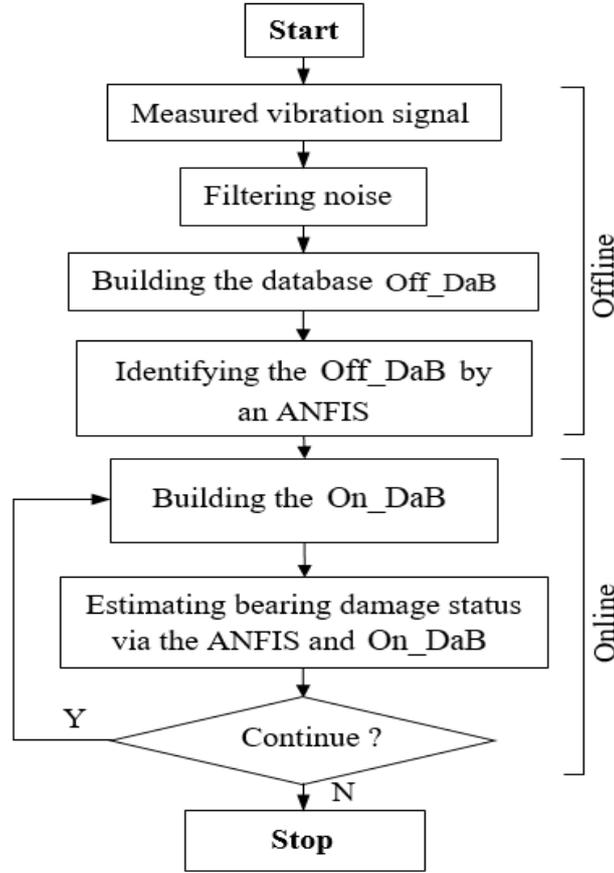
Figure 2. Flowchart of the ASBDIM
