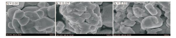
Fig. 2. SEM images of Sm doped ZnWO<sub>4</sub> nanopowders
