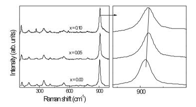
Fig. 4. Raman spectra of Sm doped  $ZnWO_4$  nanopowders. The right one is the enlarged peak of 900 cm<sup>-1</sup>.
