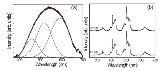
**Fig. 5.** (a) PL spectra of the ZnWO<sub>4</sub> synthesized by the hydro thermal method for 8 h (the solid lines are fitting results by using Gauss distribution); (b) Emission spectra of the Sm<sup>3+</sup> doped ZnWO<sub>4</sub> at room temperature
