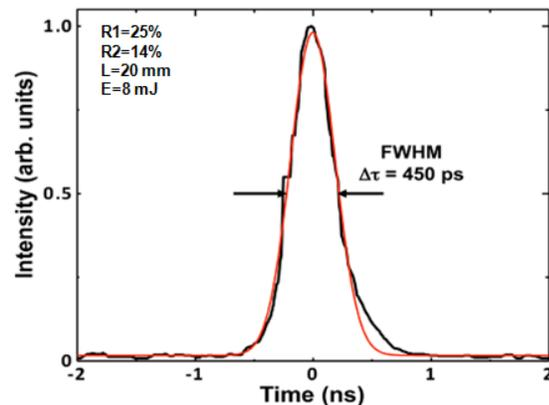
**Fig. 7.** Single 450 ps laser pulses at 290 nm were generated from the Ce:LiCAF laser by controlled resonator transient, corresponding to a pulse-shortening factor of 14 times.
