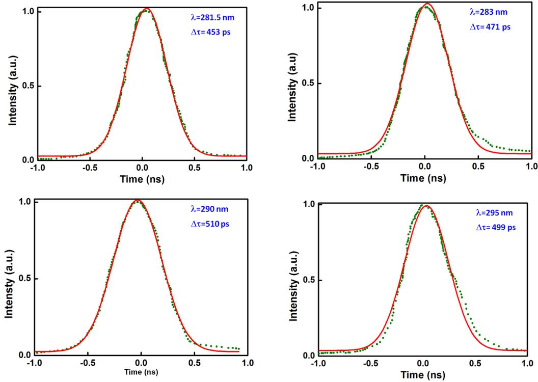
**Fig. 9.** Temporal profiles of single short (sub-nanosecond) laser pulse generated at different wavelengths at the near-threshold laser operation.
