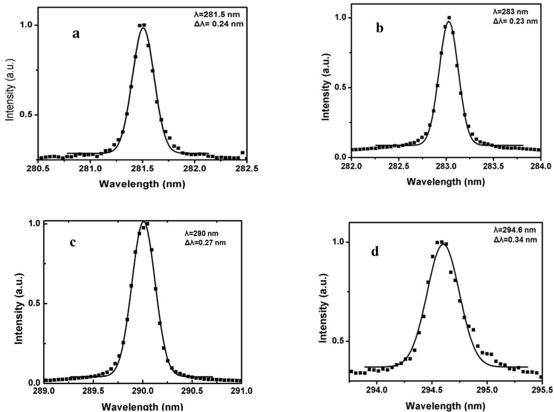
**Fig. 8.** Spectral profiles and linewidths of the tunable Ce:LiCAF laser emission for different wavelengths.
