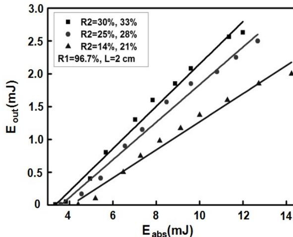
**Fig. 5.** Dependence of the laser slope efficiency on the reflectivity of the output coupler mirror ( $R_2$ ). The resonator length is 2 cm.
