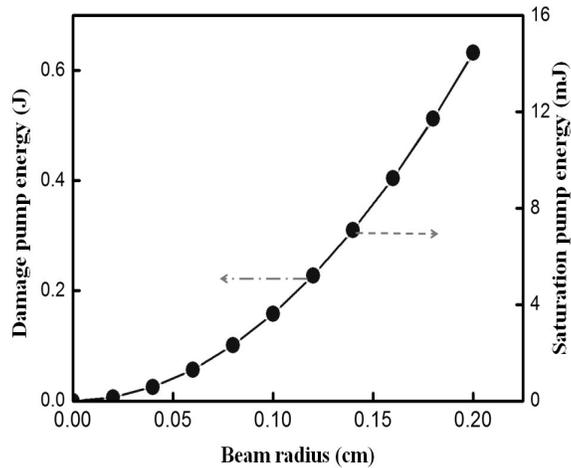
**Fig. 2.** Saturation pump and damage energy of the Ce:LiCAF crystal as a function of pumping beam radius at 266 nm pump wavelength.
