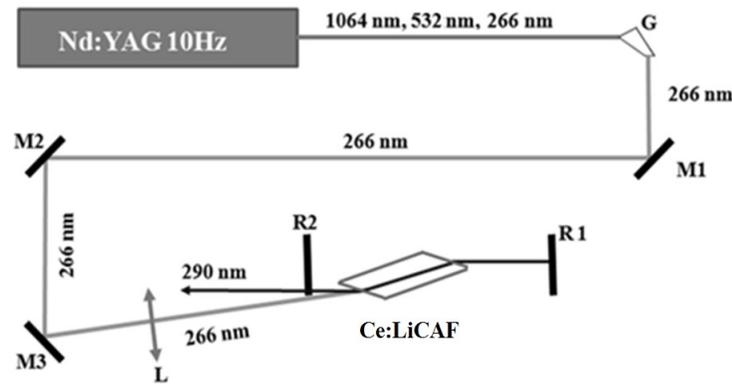
**Fig. 1.** Schematic diagram of the Ce:LiCAF laser configuration.
