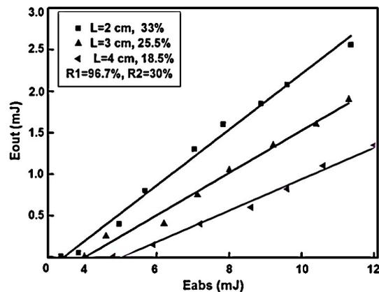
**Fig. 6.** Dependence of the laser slope efficiency on the resonator length ( $L$ ). Reflectivity of the output coupler mirror ( $R_2$ ) is 30%.
