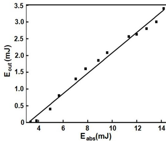
**Fig. 3.** Output energy of the broadband Ce:LiCAF laser emission as a function of absorbed pump energy. The laser slope efficiency is 33%.
