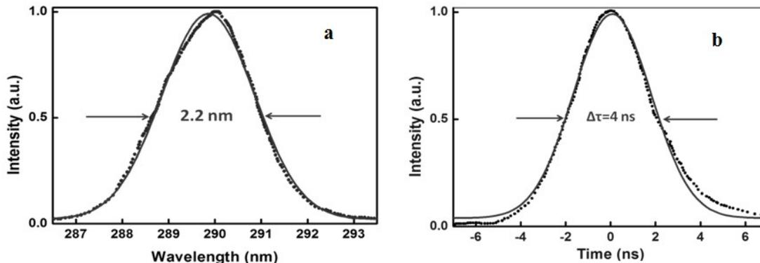
**Fig. 4.** (a) Spectral and (b) temporal profiles of the broadband Ce:LiCAF laser output from the resonator having 96.7% end mirror reflectivity, 30% output coupler reflectivity, 2 cm resonator length and 10 mJ pump energy pulses.
