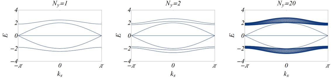
**Fig. 2.** (Color online) The evolution of the band structure with increasing  $N_y$ . The model parameters  $\lambda = 0.4$ ,  $\delta = 0$ ,  $h_A = h_B = h_C = 0$  are chosen as an example.
