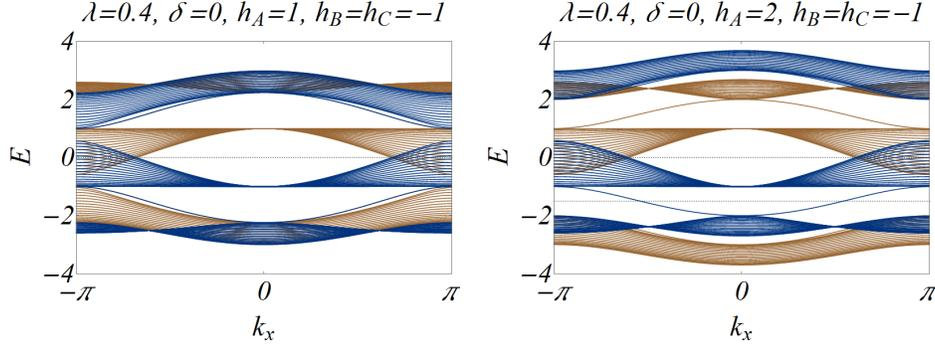
**Fig. 8.** (Color online) The band structure with different magnetic fields  $0 < h_A < h_B = h_C$  at fixed SOC in the absence of the lattice modulation. Brown (blue) color represents the band structure for the spin up (down) component. The dotted lines show a position of the chemical potential at half and third fillings.
