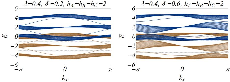
**Fig. 10.** (Color online) The band structure with different lattice modulations  $\delta$  at fixed SOC and strong  $h_A = h_B = h_C$ . Brown (blue) color represents the band structure for the spin up (down) component. The dotted lines show a position of the chemical potential at half, third and sixth fillings.
