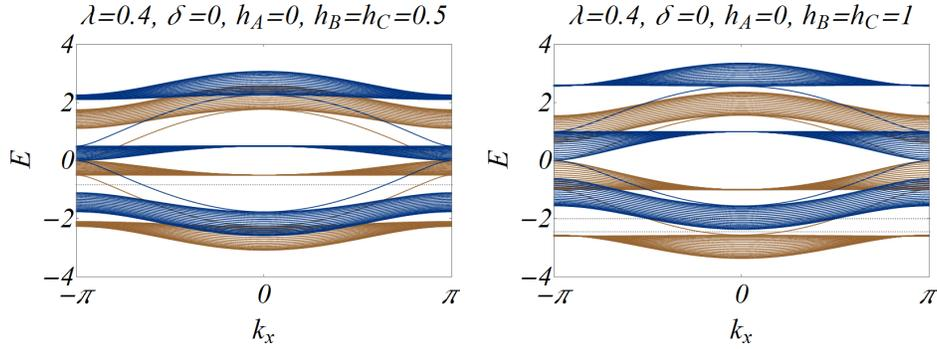
**Fig. 5.** (Color online) The band structure with different magnetic fields  $h_A = 0, h_B = h_C \neq 0$  at fixed SOC in the absence of the lattice modulation. Brown (blue) color represents the band structure for the spin up (down) component. The dotted lines show a position of the chemical potential at third filling (left panel) and at sixth and slightly larger sixth fillings (right panel).
