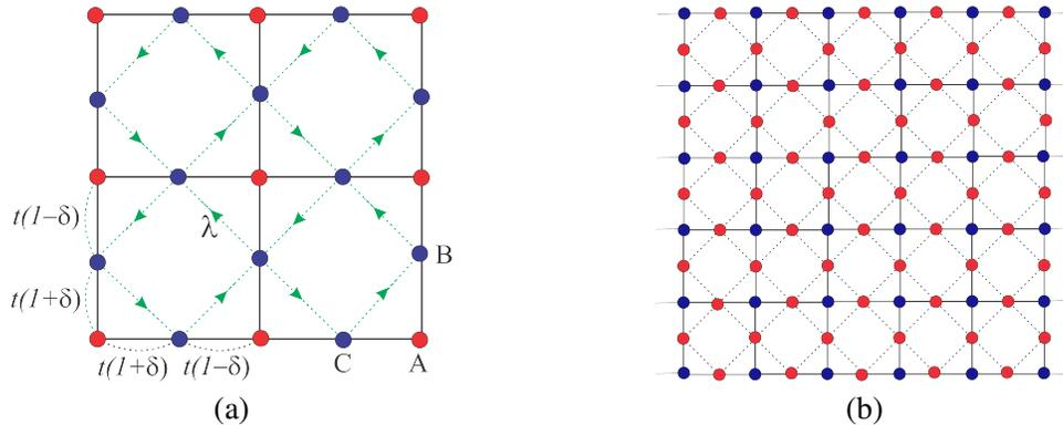
**Fig. 1.** (a) The Lieb lattice structure with SOC and lattice modulation. The arrows indicate the sign  $v_{ij} = 1$  of the SOC. In the opposite direction  $v_{ij} = -1$ . (b) A nano-ribbon with straight-straight open boundaries in the  $y$ -axis and periodic boundaries in the  $x$ -axis.
