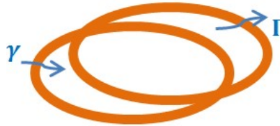
Fig. 1. Schematic show of the double ring structure with linear gain \gamma and nonlinear loss \Gamma
