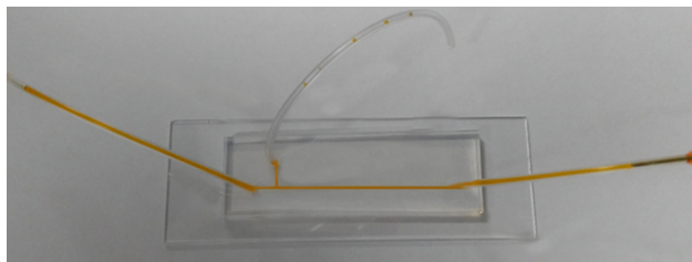
Fig. 4. Test the bonding between PDMS channel and glass substrate.
