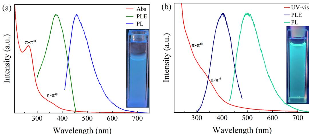
**Fig. 3.** (Color online) UV-vis absorption, Normalized PLE, and PL spectra ( $\lambda_{\text{ex}} = 405$  nm) of (a) B-CQDs, (b) G-CQDs.
