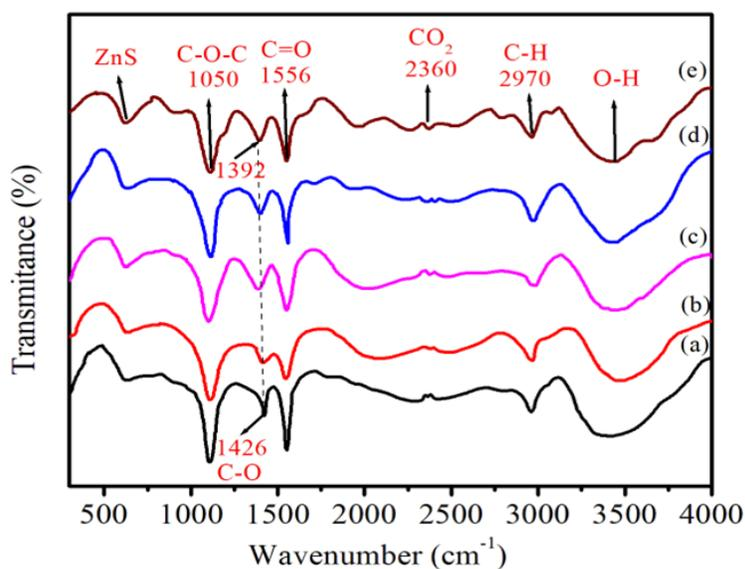
**Fig. 3.** FT-IR spectra of the NCs: ZnS (a), ZnS:Dy<sup>3+</sup>0.5% (b), ZnS:Dy<sup>3+</sup>1% (c), ZnS:Dy<sup>3+</sup>2% (d), and ZnS:Dy<sup>3+</sup>3% (e).
