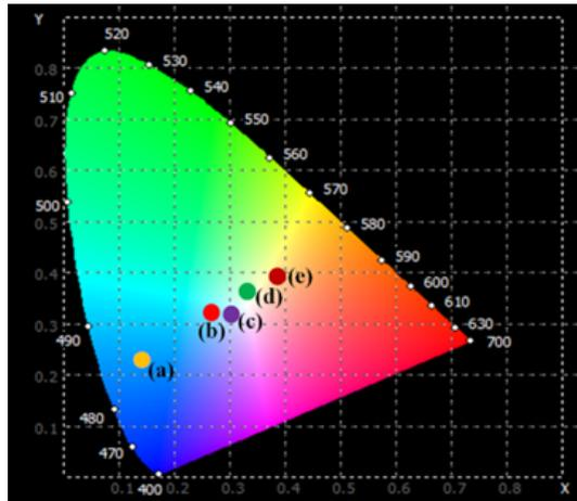
**Fig. 7.** CIE color coordinates of Dy<sup>3+</sup>-doped ZnS NCs at  $\lambda_{\text{exc}} = 350$  nm.
