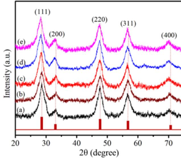
**Fig. 1.** X-ray diffraction pattern of: ZnS (a), ZnS:Dy<sup>3+</sup>0.5% (b), ZnS:Dy<sup>3+</sup>1% (c), ZnS:Dy<sup>3+</sup>2% (d), and ZnS:Dy<sup>3+</sup>3% (e).
