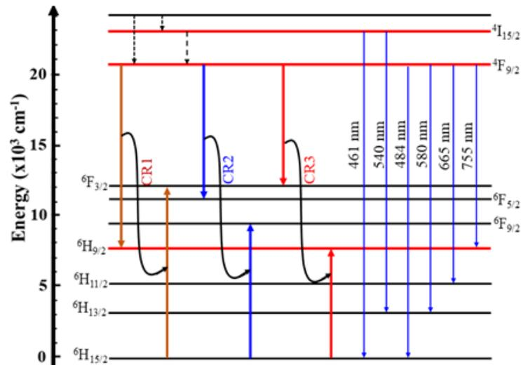
**Fig. 6.** Energy band structure and energy transfer channels in ZnS: Dy<sup>3+</sup> NCs.
