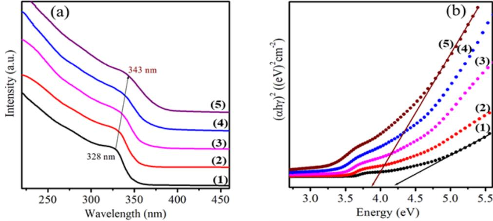
**Fig. 4.** (a) UV-vis spectra of NCs: ZnS (1), ZnS:Dy<sup>3+</sup>0.5% (2), ZnS:Dy<sup>3+</sup>1% (3), ZnS:Dy<sup>3+</sup>2% (4), and ZnS:Dy<sup>3+</sup>3% (5); (b) Dependence of  $(\alpha hv)^2$  on energy ( $h\nu$ ) of Dy<sup>3+</sup>-doped ZnS NCs.
