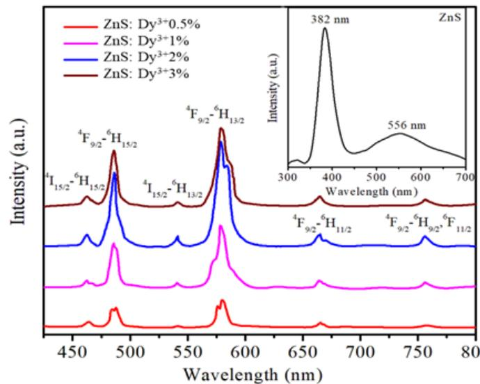
**Fig. 5.** PL spectra of Dy<sup>3+</sup>-doped ZnS NCs under 350 nm excitation wavelength.
