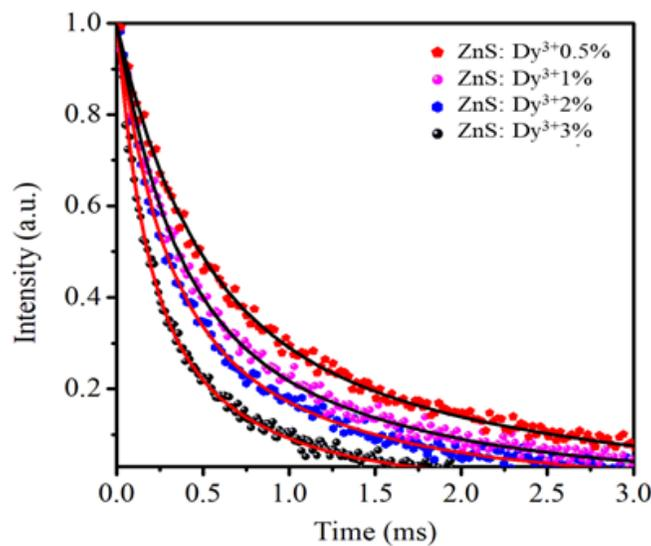
**Fig. 8.** (Color online) Time-resolved fluorescence curves of Dy<sup>3+</sup>-doped ZnS NCs measured at 580 nm (4F<sub>9/2</sub> → 6H<sub>13/2</sub>).
