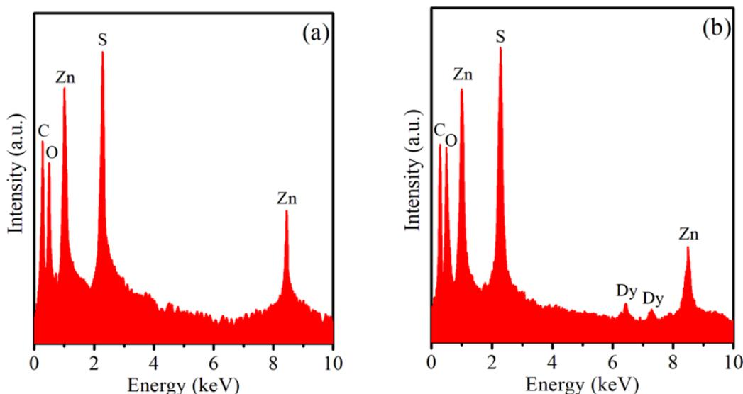
**Fig. 2.** EDX spectra of ZnS (a) and ZnS: Dy<sup>3+</sup> 3% (b) NCs.
